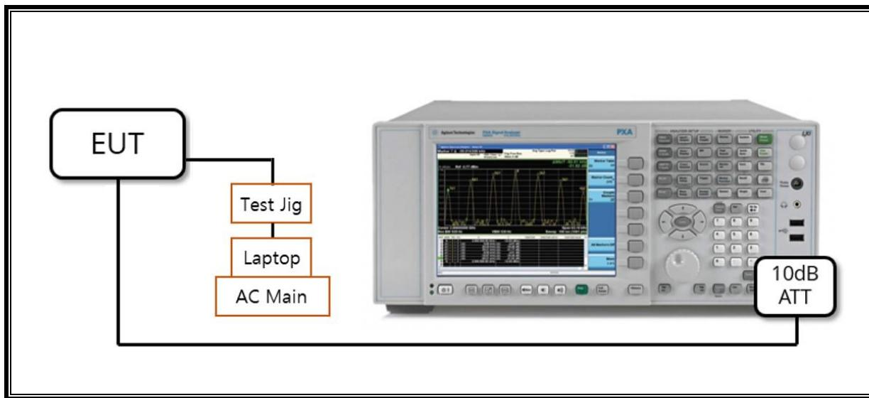
**SETUP DIAGRAM FOR TESTS (RADIATED TEST SETUP)**
