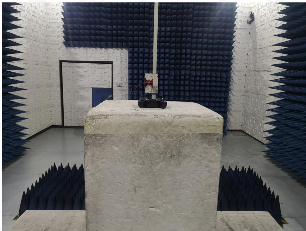
FCC RADIATED EMISSION TEST SETUP ABOVE 1GHZ
