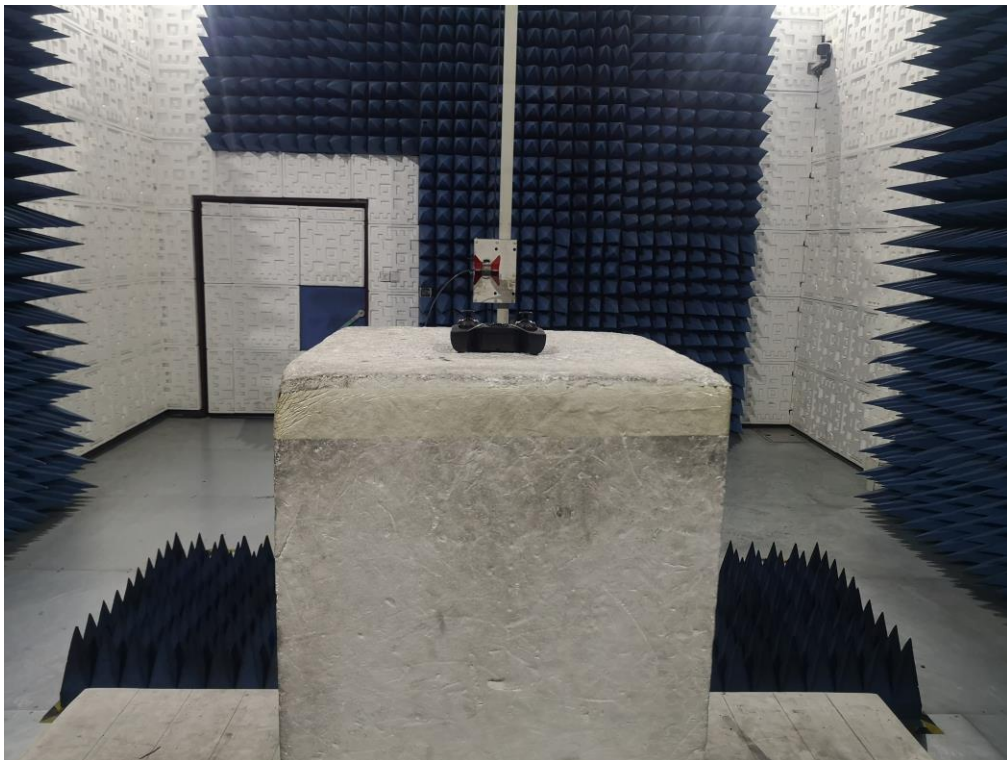
FCC RADIATED EMISSION TEST SETUP ABOVE 1GHZ
