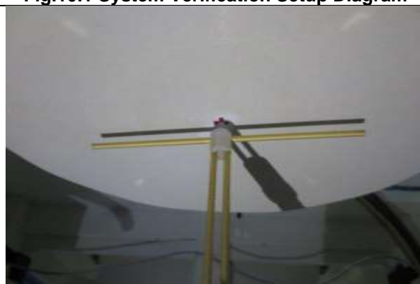
Fig.10.2 Photo of Dipole setup
