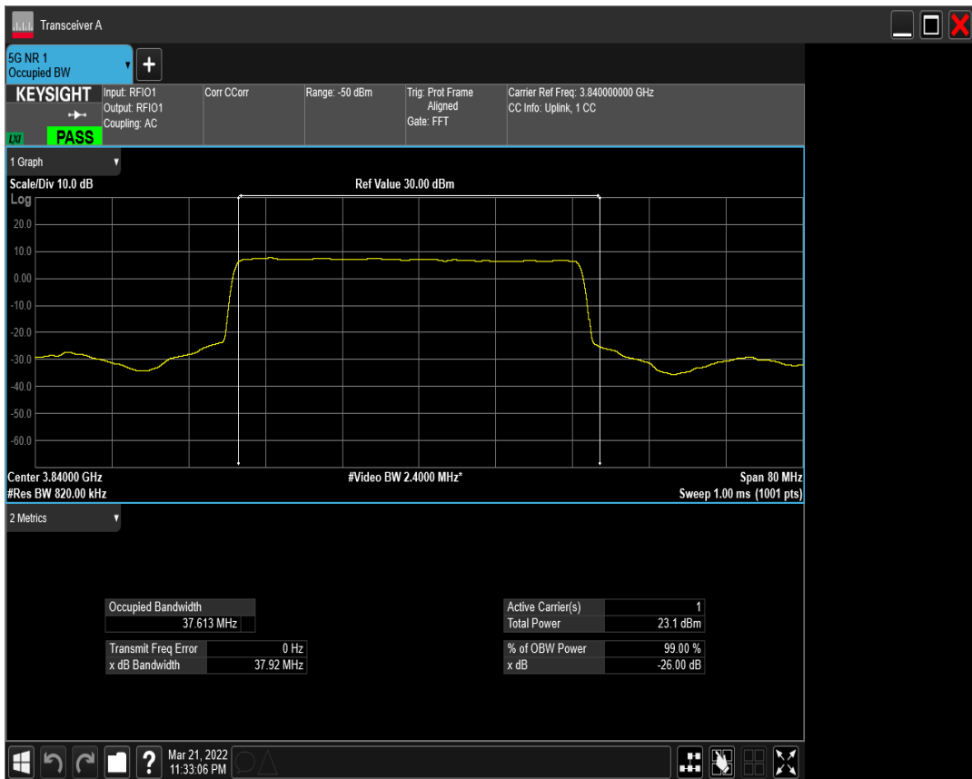
n77(3700-3980) SCS=30kHz DFT_QPSK BW=40MHz Channel=656000 RB=100@0
