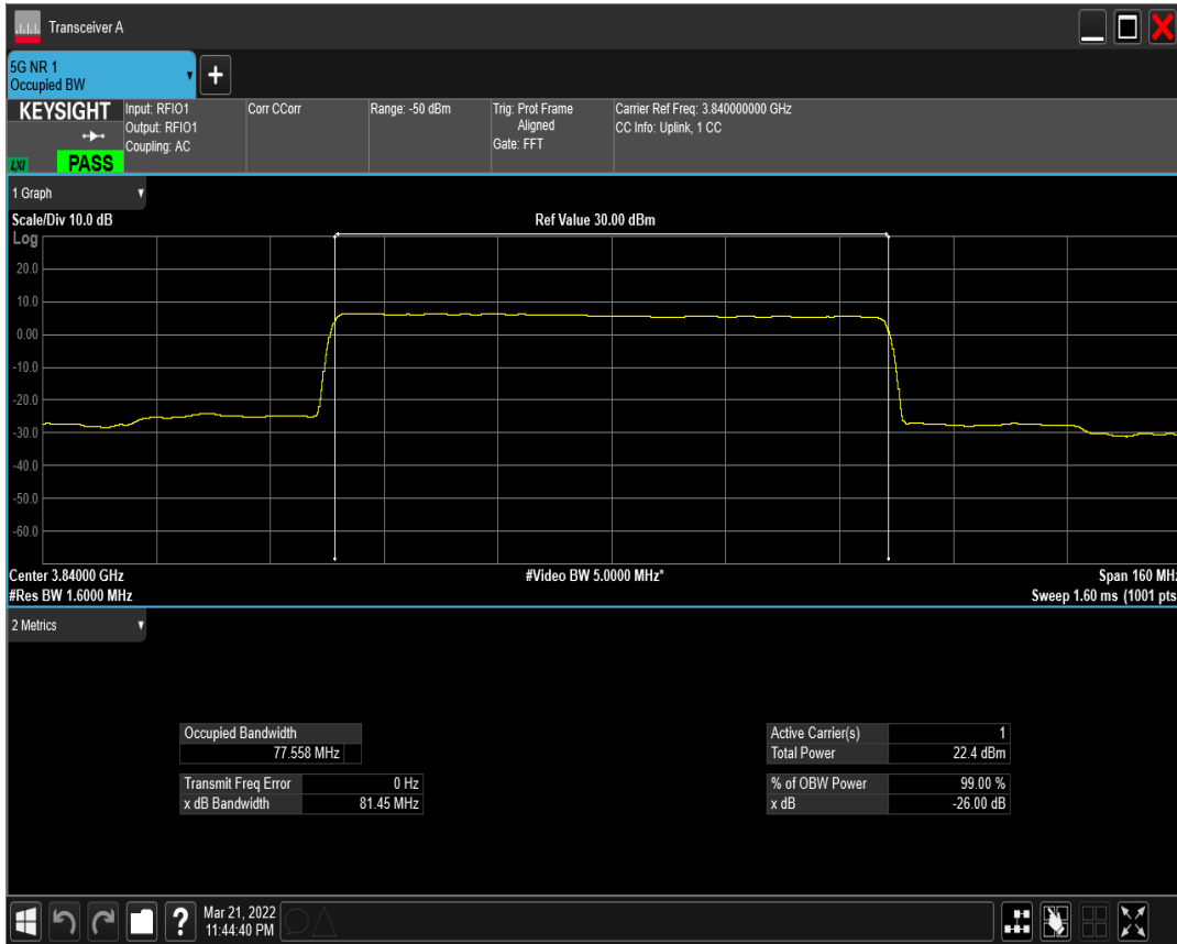
n77(3700-3980) SCS=30kHz DFT_QAM16 BW=80MHz Channel=656000 RB=216@0
