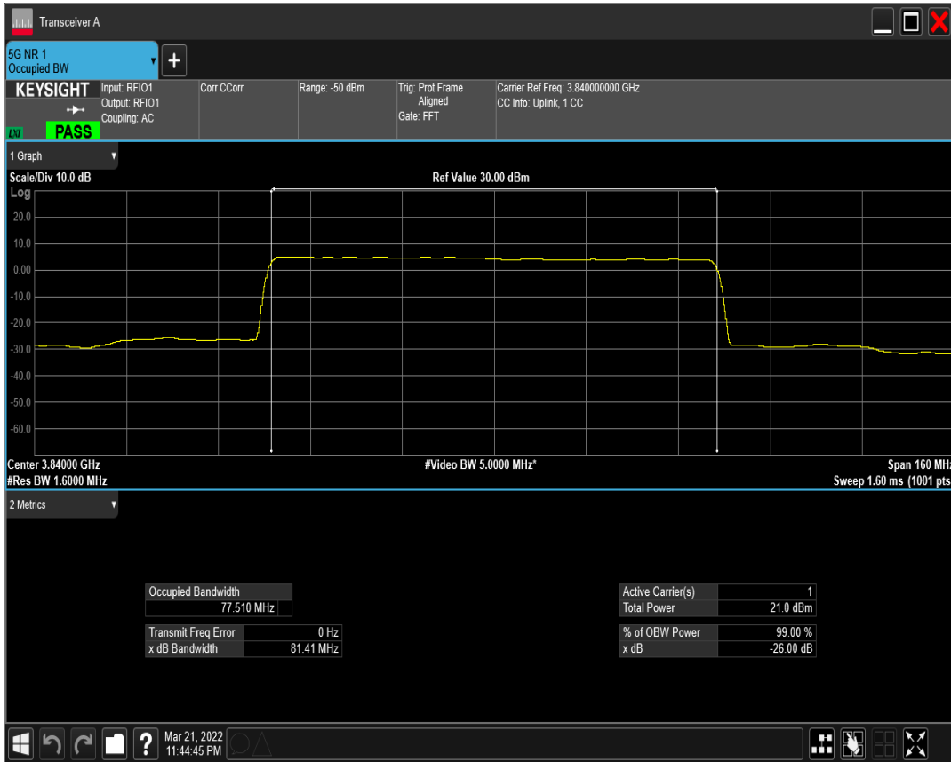
n77(3700-3980) SCS=30kHz DFT_QAM256 BW=80MHz Channel=656000 RB=216@0
