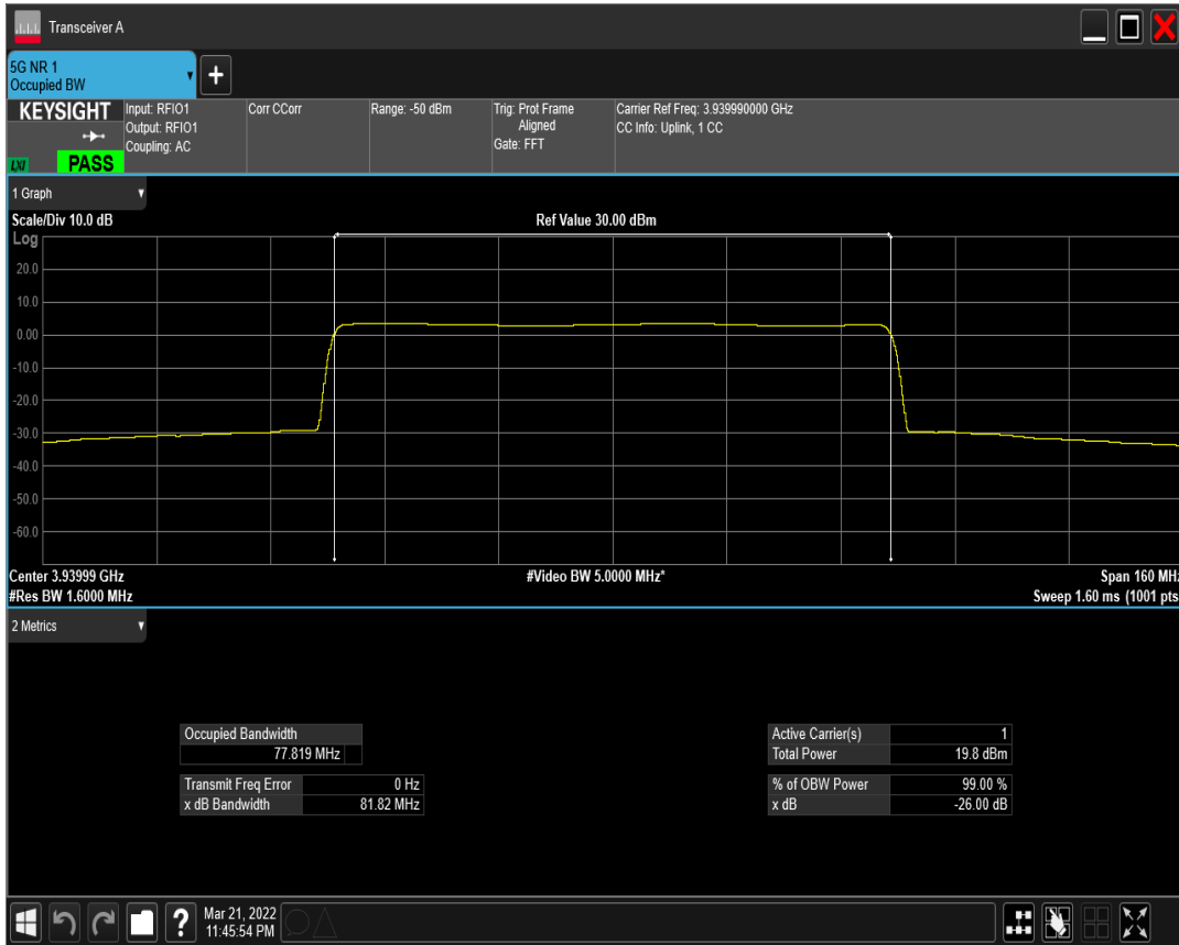
n77(3700-3980) SCS=30kHz DFT_BPSK BW=90MHz Channel=649668 RB=240@0
