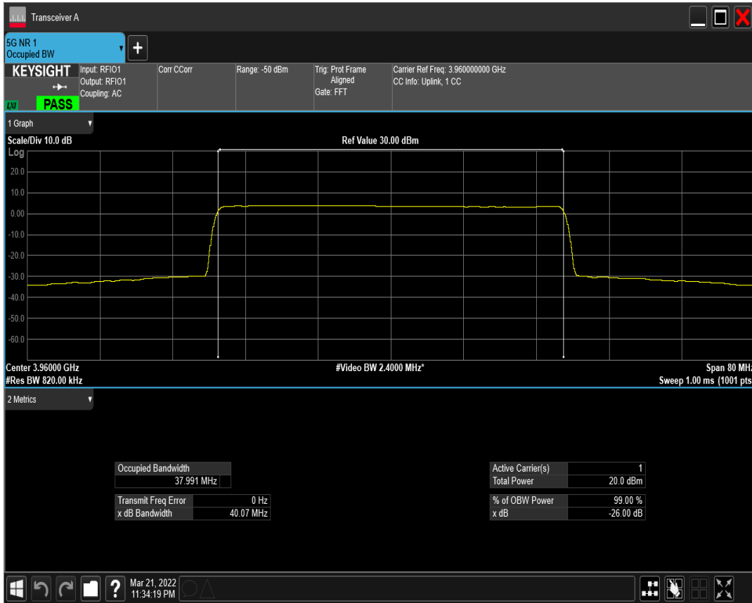
n77(3700-3980) SCS=30kHz DFT_BPSK BW=50MHz Channel=648334 RB=128@0
