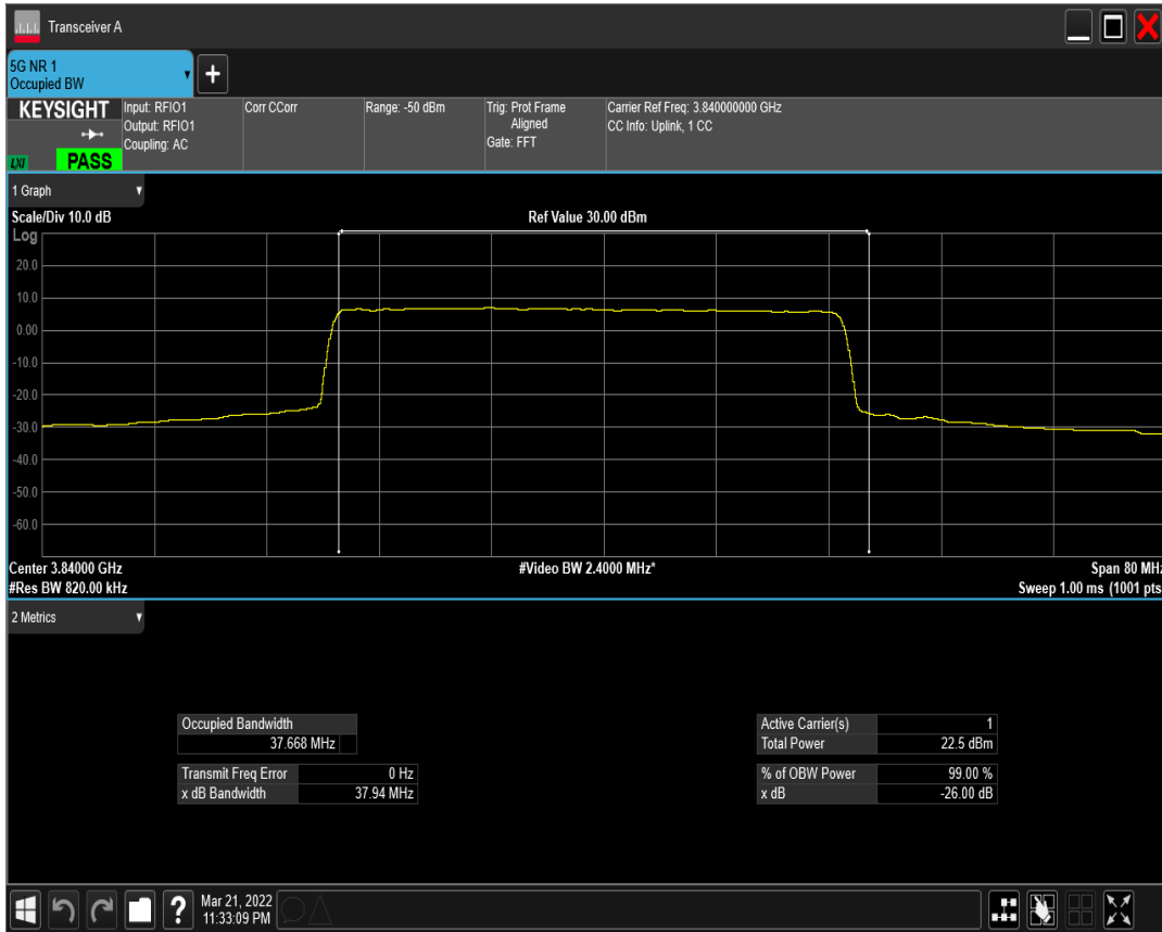
n77(3700-3980) SCS=30kHz DFT_QAM16 BW=40MHz Channel=656000 RB=100@0
