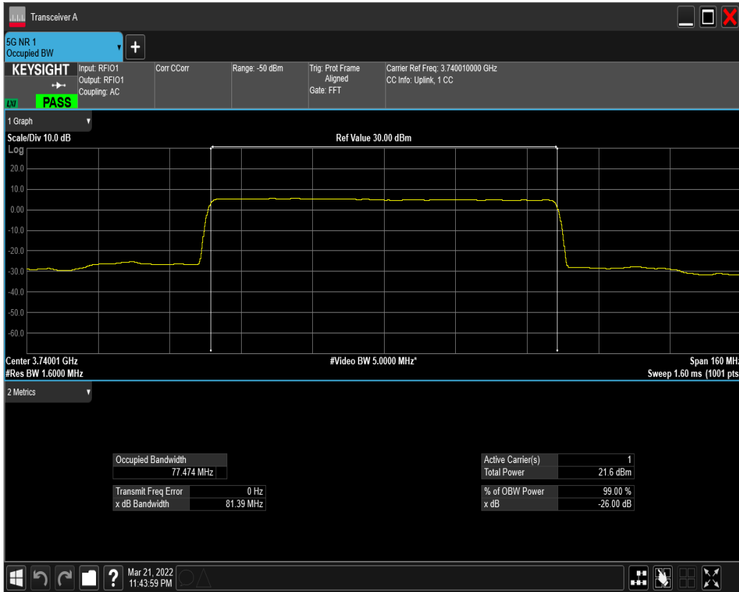
n77(3700-3980) SCS=30kHz DFT_QAM256 BW=80MHz Channel=649334 RB=216@0
