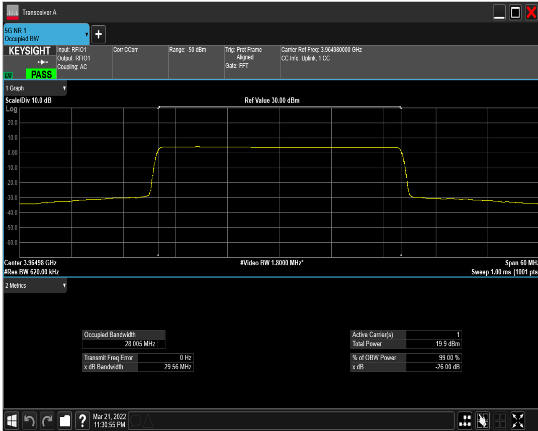
n77(3700-3980) SCS=30kHz DFT_BPSK BW=40MHz Channel=648000 RB=100@0
