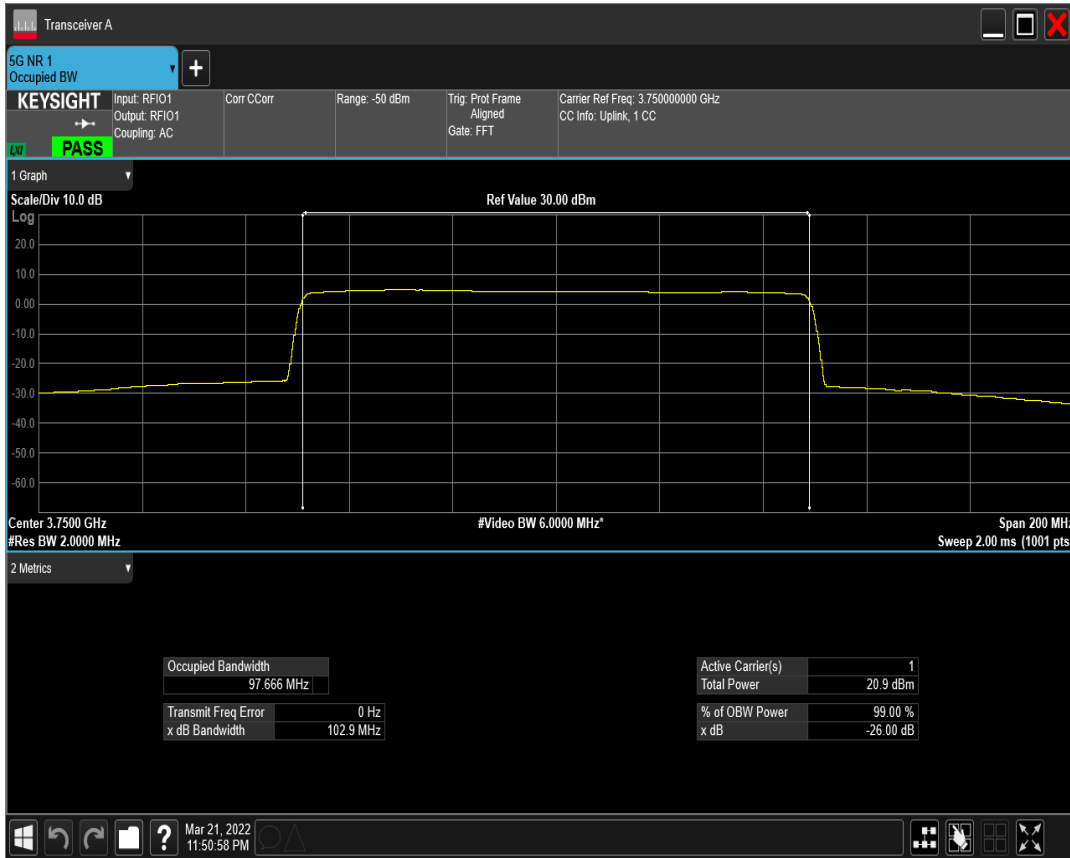
n77(3700-3980) SCS=30kHz DFT_BPSK BW=100MHz Channel=656000 RB=270@0
