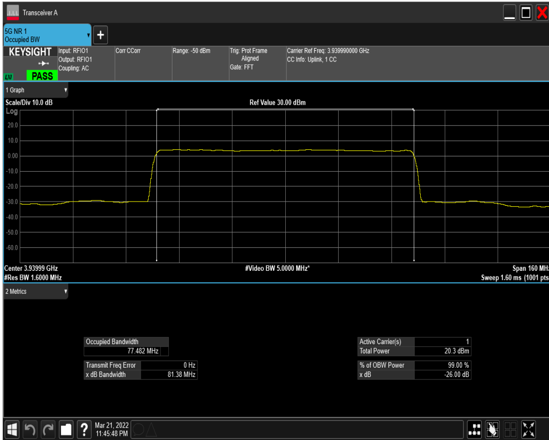
n77(3700-3980) SCS=30kHz DFT_QAM256 BW=80MHz Channel=662666 RB=216@0
