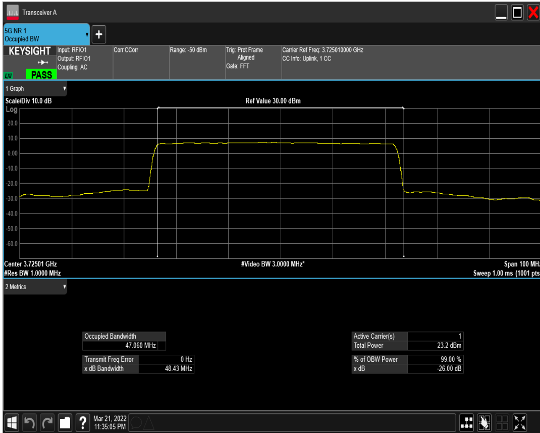
n77(3700-3980) SCS=30kHz DFT_QAM16 BW=50MHz Channel=648334 RB=128@0
