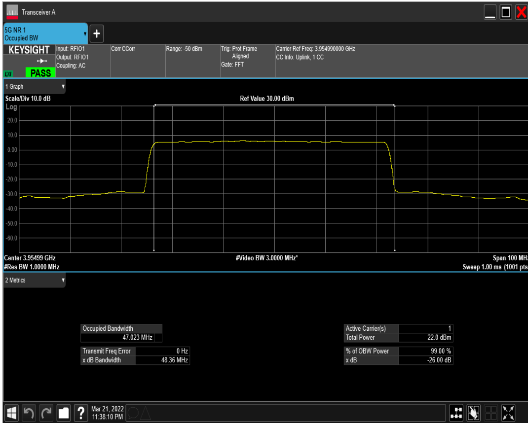
n77(3700-3980) SCS=30kHz DFT_QAM16 BW=50MHz Channel=663666 RB=128@0
