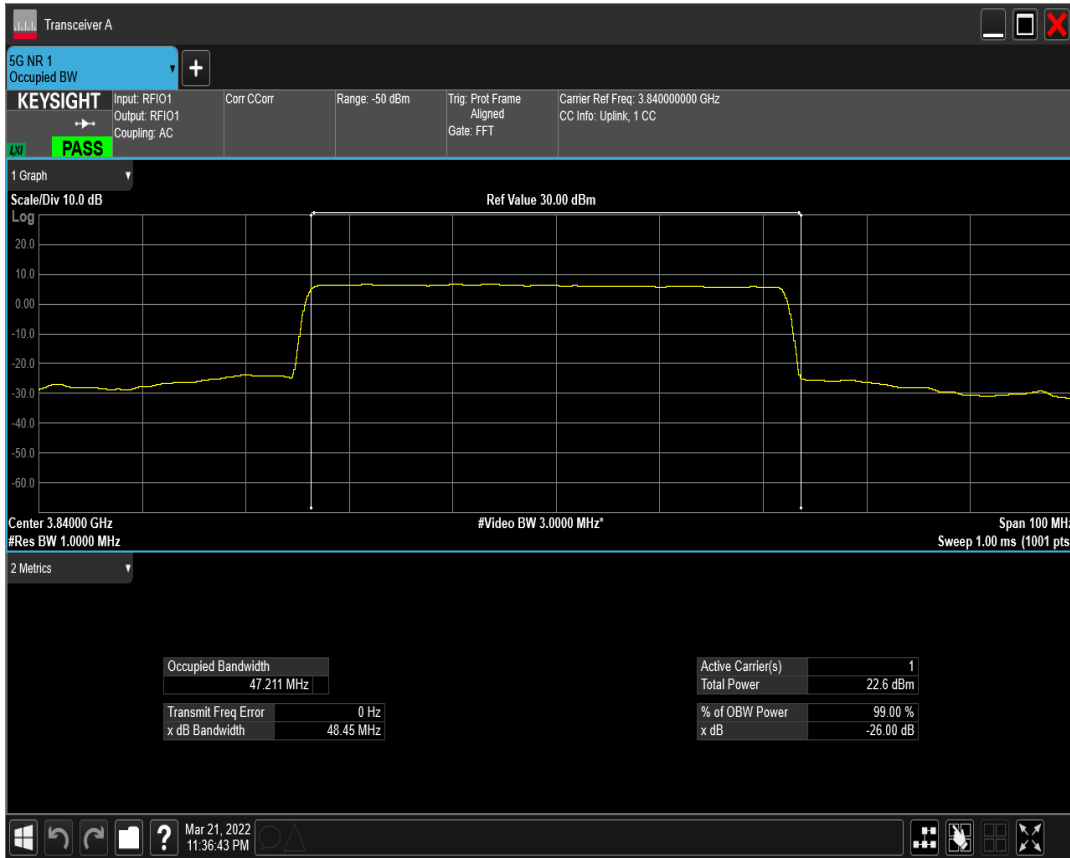
n77(3700-3980) SCS=30kHz DFT_QAM16 BW=50MHz Channel=656000 RB=128@0
