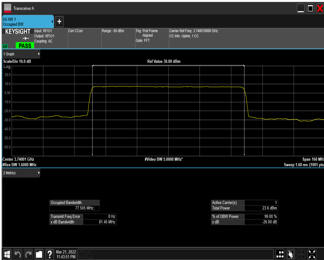
n77(3700-3980) SCS=30kHz DFT_QPSK BW=80MHz Channel=649334 RB=216@0
