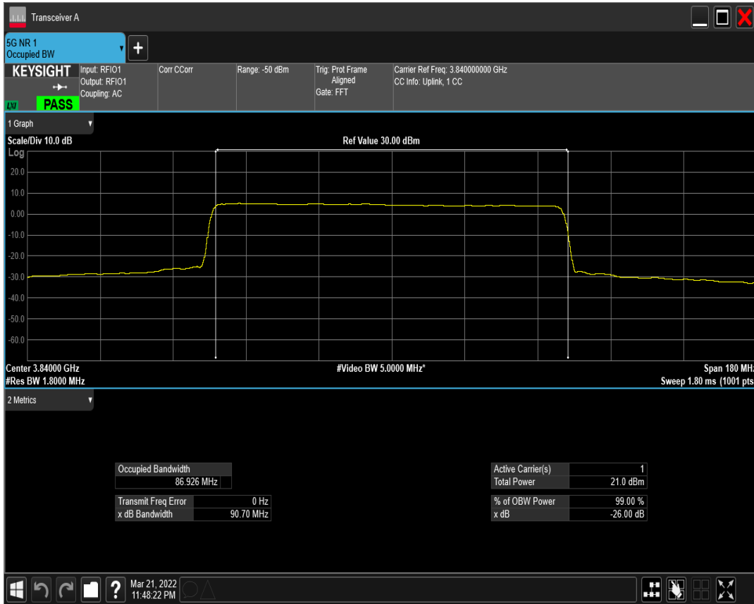
n77(3700-3980) SCS=30kHz DFT_QAM256 BW=90MHz Channel=656000 RB=240@0
