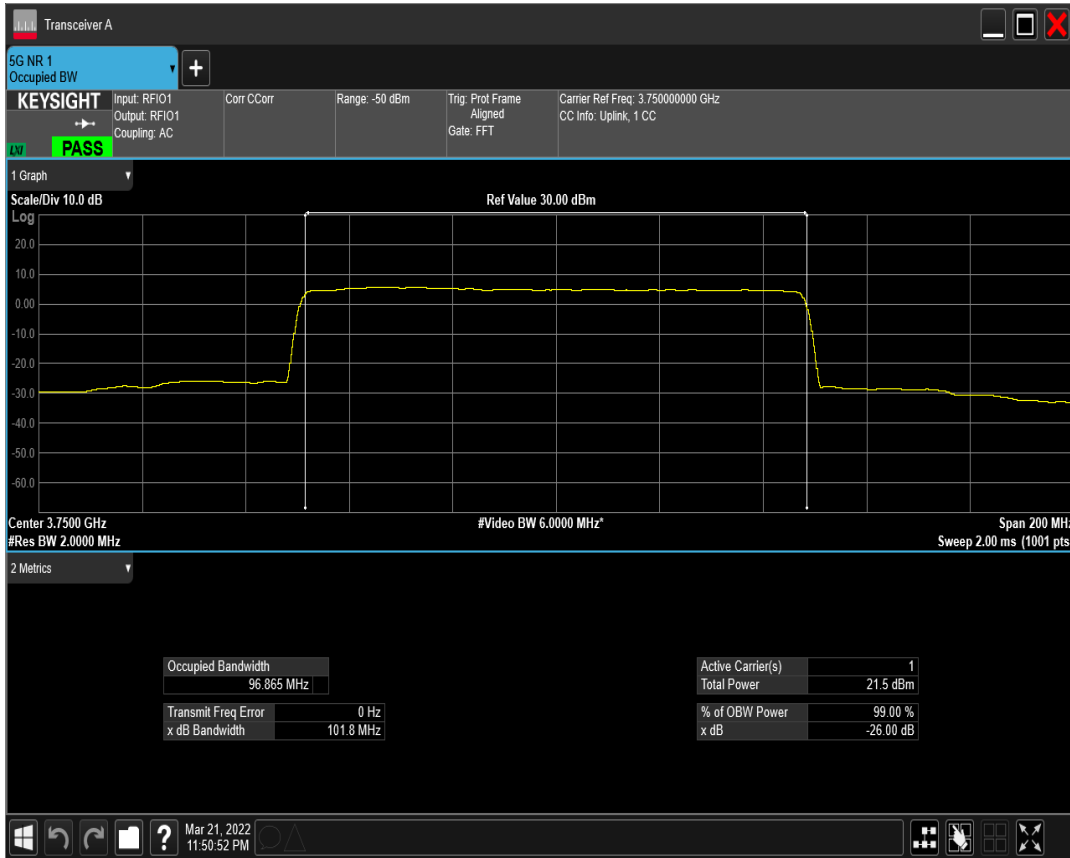
n77(3700-3980) SCS=30kHz DFT_QAM256 BW=100MHz Channel=650000 RB=270@0
