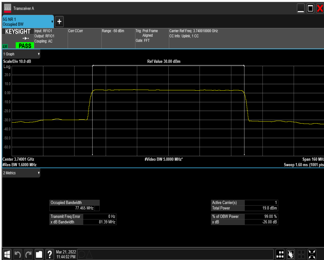
n77(3700-3980) SCS=30kHz CP_QPSK BW=80MHz Channel=649334 RB=217@0
