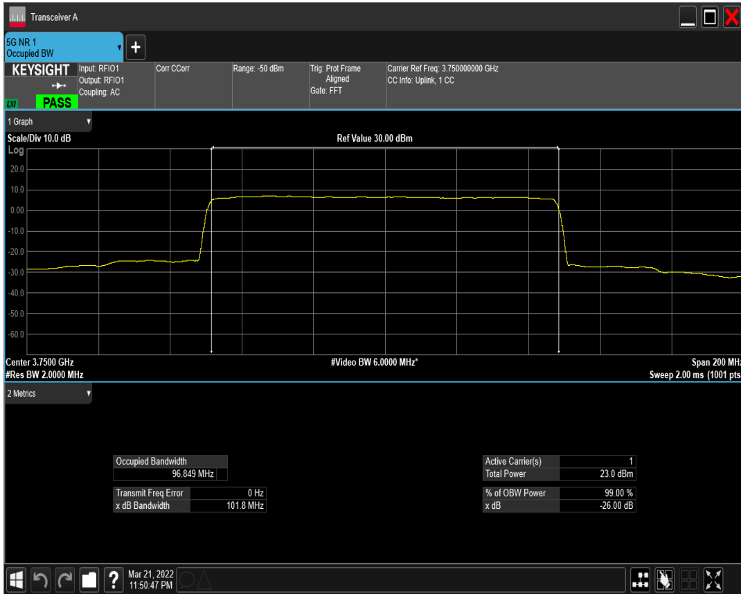
n77(3700-3980) SCS=30kHz DFT_QAM16 BW=100MHz Channel=650000 RB=270@0
