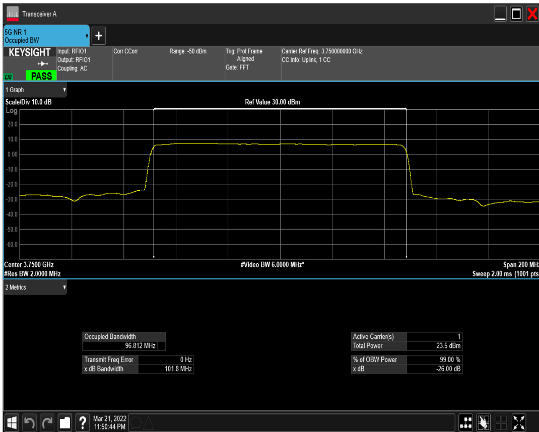
n77(3700-3980) SCS=30kHz DFT_QPSK BW=100MHz Channel=650000 RB=270@0
