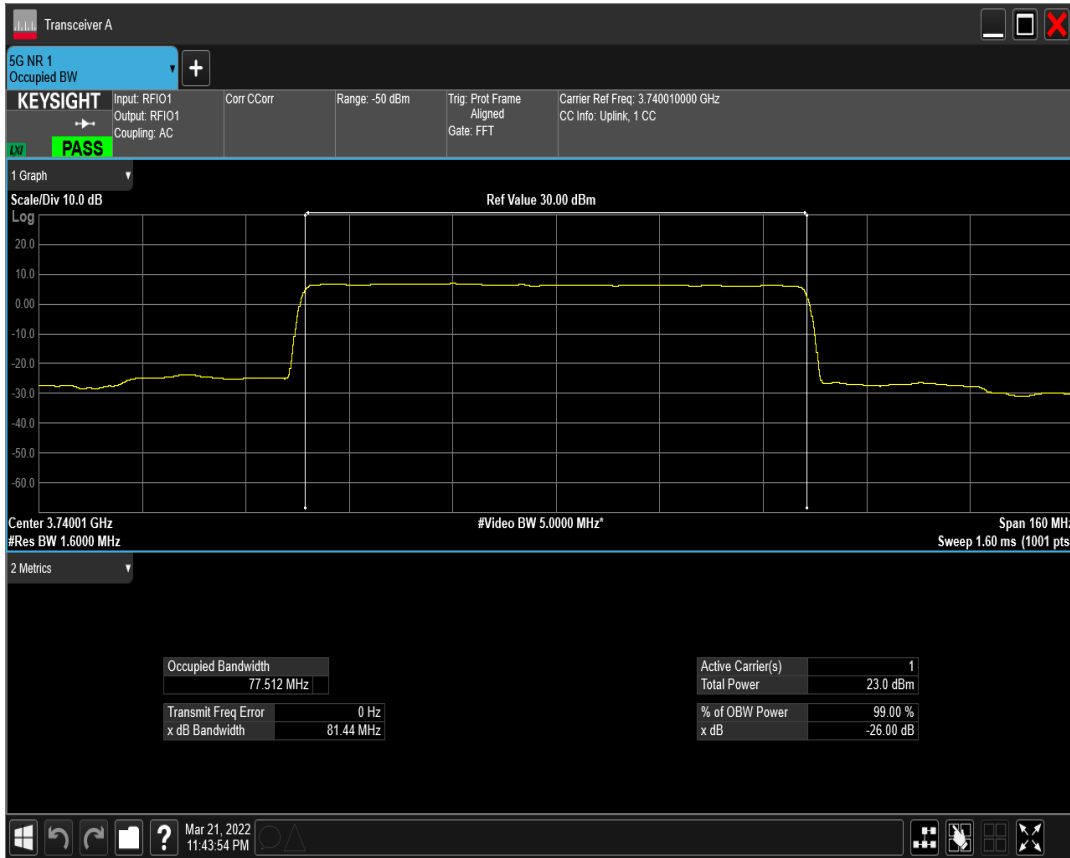
n77(3700-3980) SCS=30kHz DFT_QAM16 BW=80MHz Channel=649334 RB=216@0
