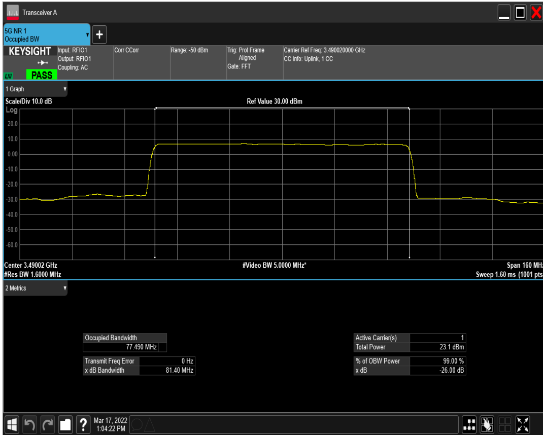
n77(3450-3550) SCS=30kHz DFT_QAM64 BW=80MHz Channel=632668 RB=216@0
