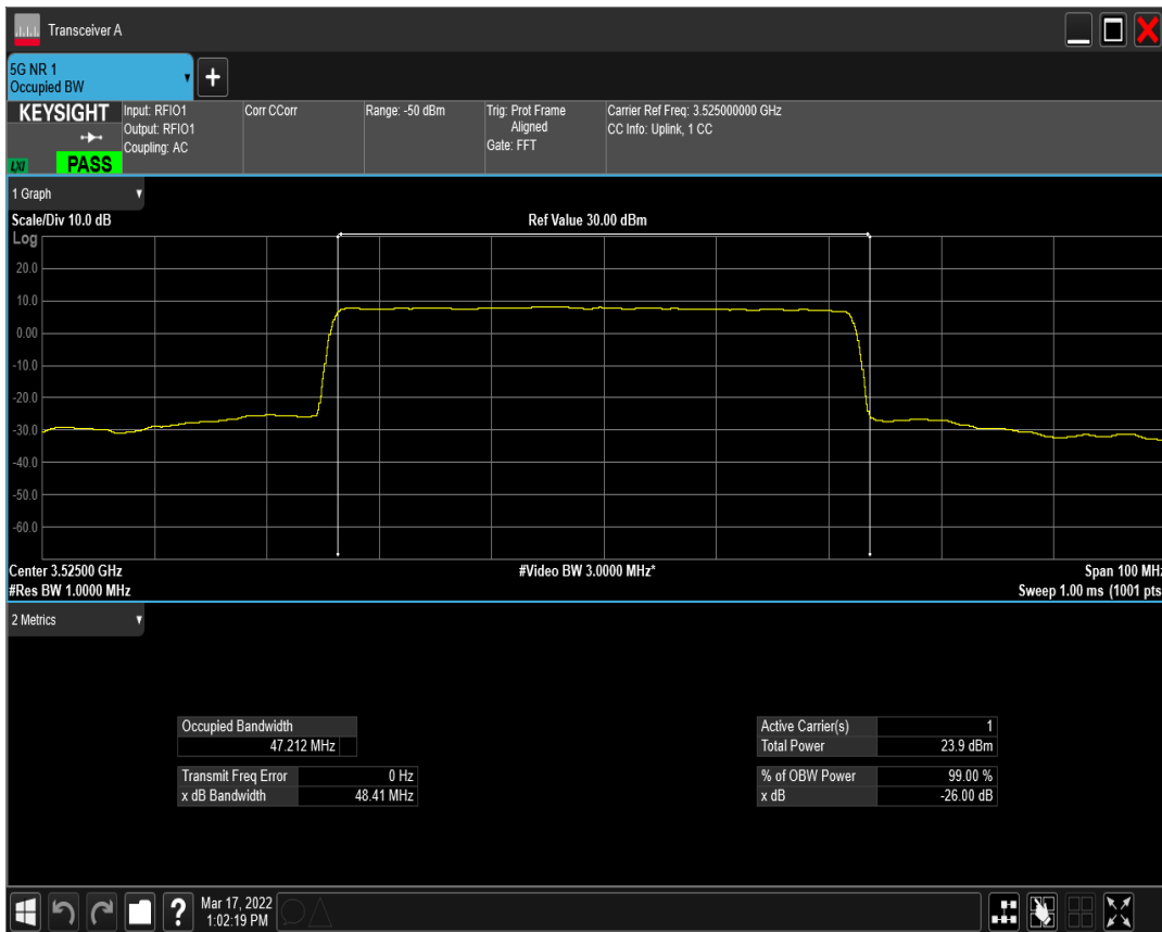
n77(3450-3550) SCS=30kHz DFT_QAM16 BW=50MHz Channel=635000 RB=128@0
