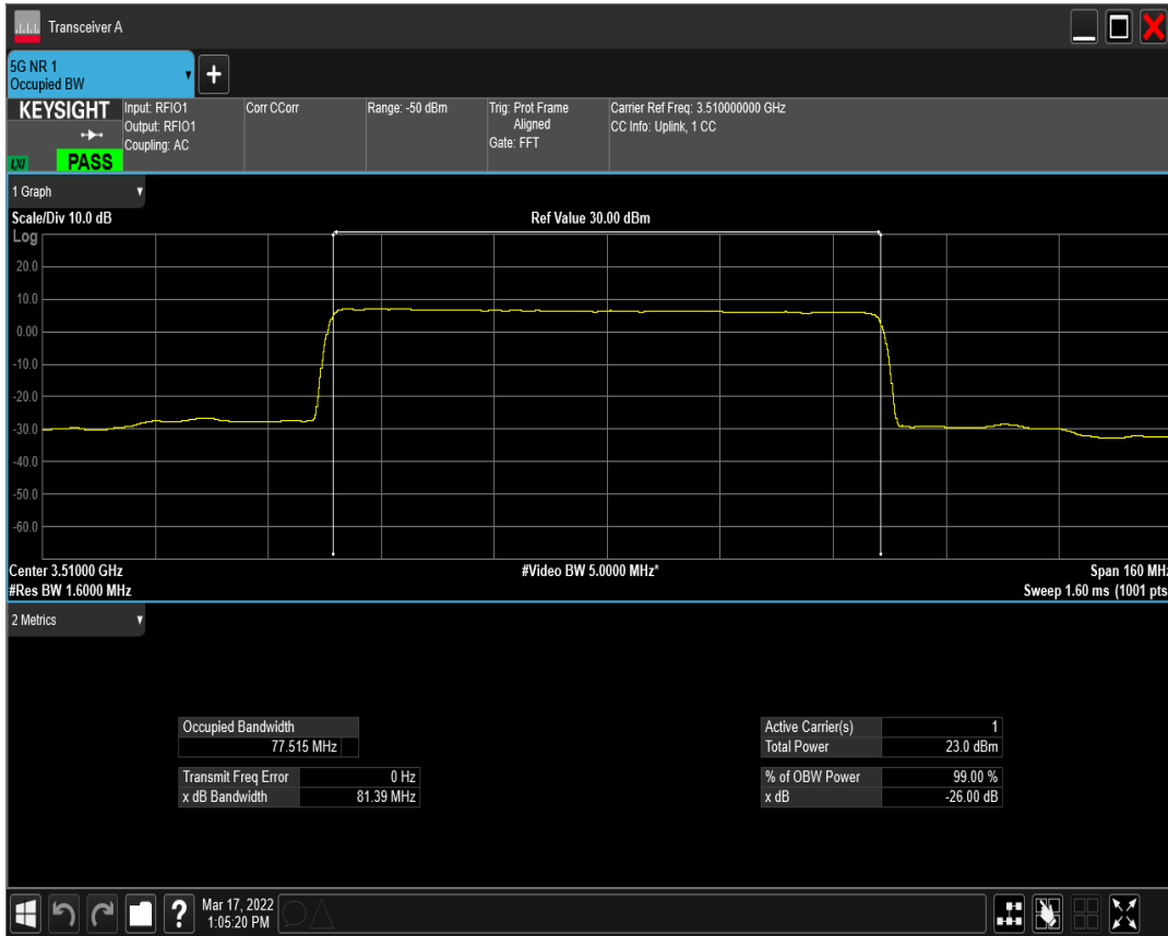
n77(3450-3550) SCS=30kHz DFT_QAM64 BW=80MHz Channel=634000 RB=216@0
