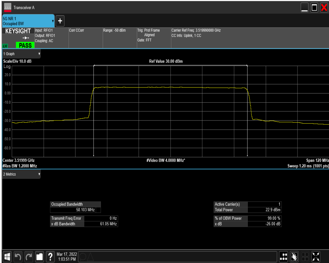
n77(3450-3550) SCS=30kHz DFT_QAM64 BW=60MHz Channel=634666 RB=162@0
