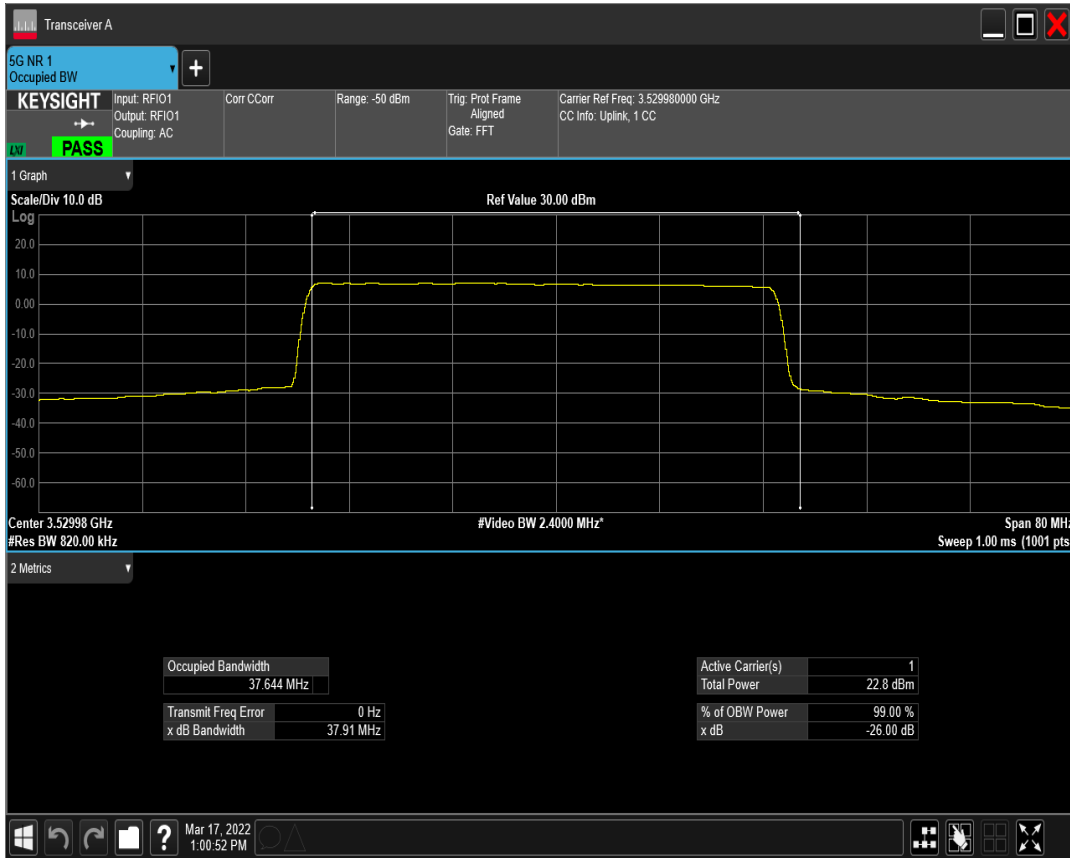
n77(3450-3550) SCS=30kHz DFT_QAM64 BW=40MHz Channel=635332 RB=100@0
