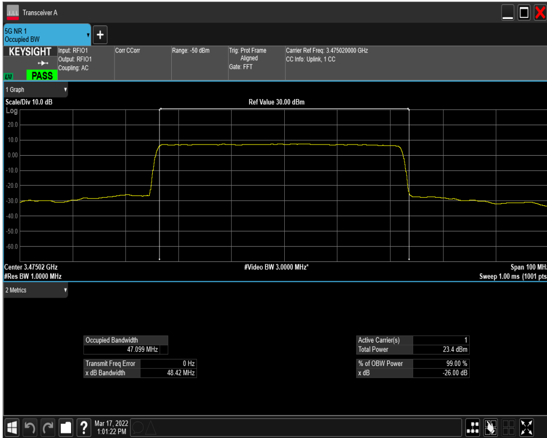
n77(3450-3550) SCS=30kHz DFT_QAM64 BW=50MHz Channel=631668 RB=128@0
