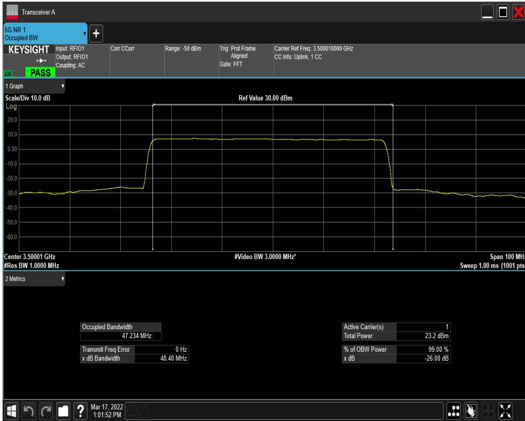
n77(3450-3550) SCS=30kHz DFT_QAM64 BW=50MHz Channel=633334 RB=128@0
