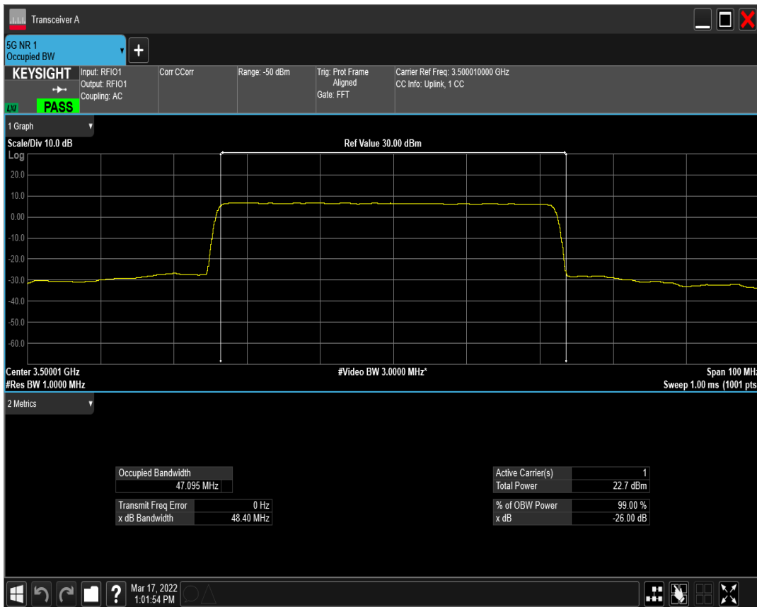
n77(3450-3550) SCS=30kHz DFT_QAM256 BW=50MHz Channel=633334 RB=128@0
