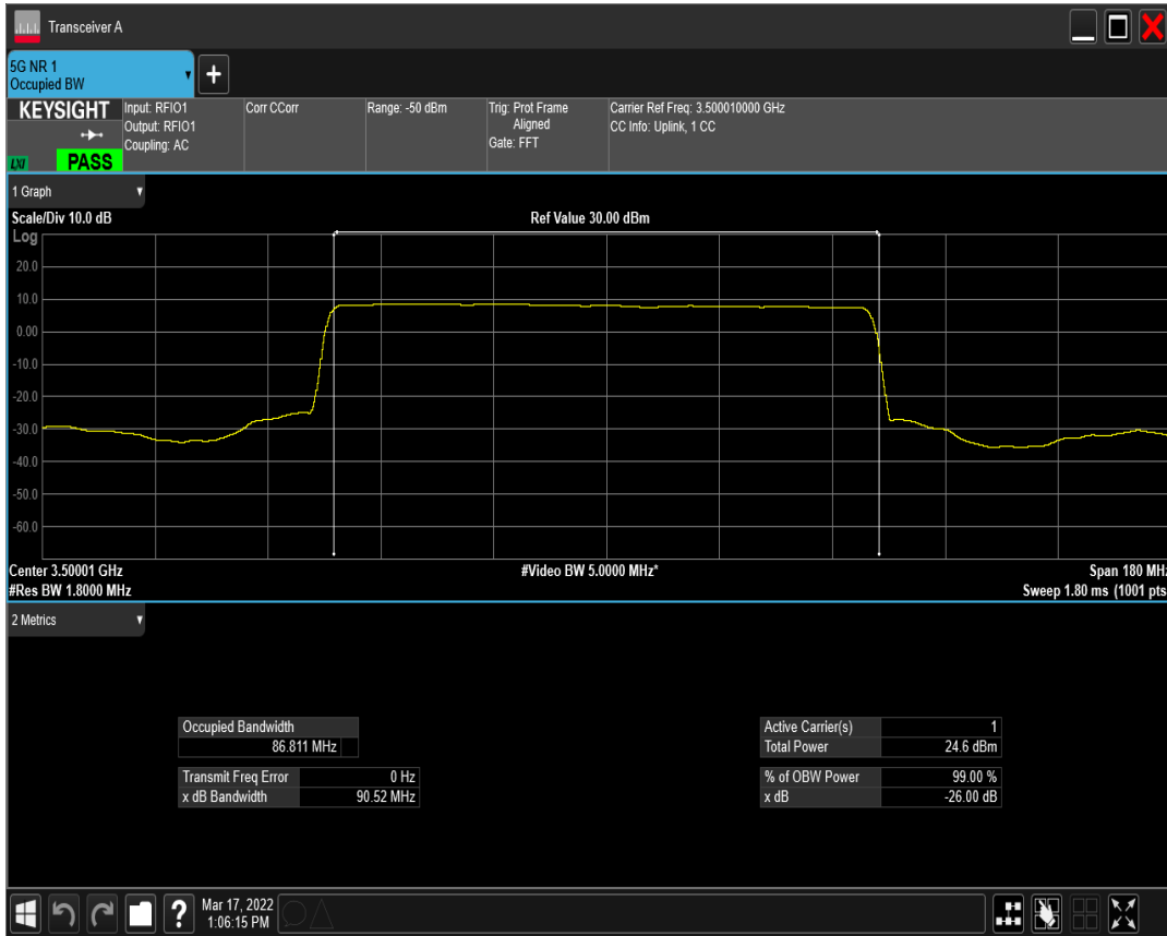
n77(3450-3550) SCS=30kHz DFT_QPSK BW=90MHz Channel=633334 RB=240@0
