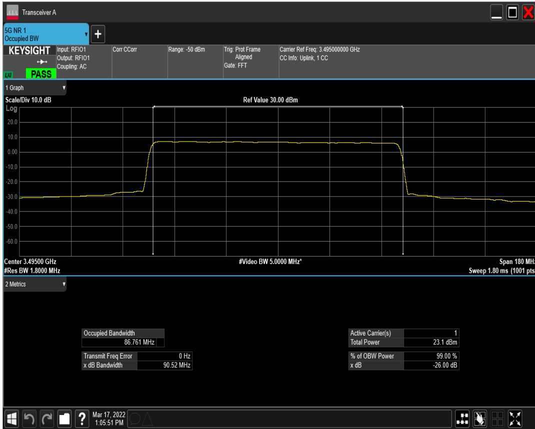
n77(3450-3550) SCS=30kHz DFT_QAM64 BW=90MHz Channel=633000 RB=240@0
