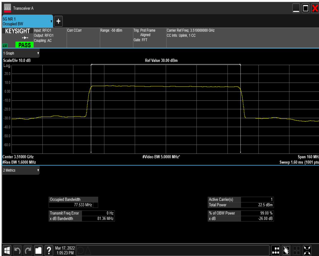
n77(3450-3550) SCS=30kHz DFT_QAM256 BW=80MHz Channel=634000 RB=216@0
