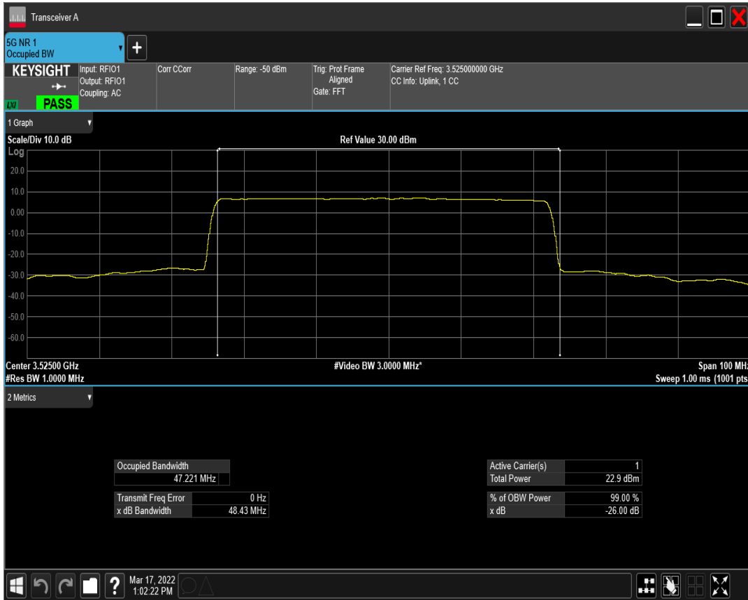
n77(3450-3550) SCS=30kHz DFT_QAM64 BW=50MHz Channel=635000 RB=128@0
