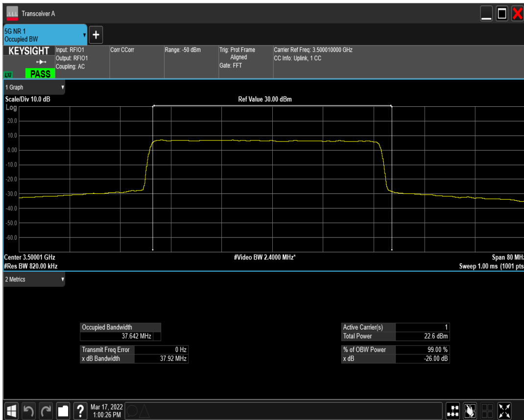
n77(3450-3550) SCS=30kHz DFT_QAM256 BW=40MHz Channel=633334 RB=100@0
