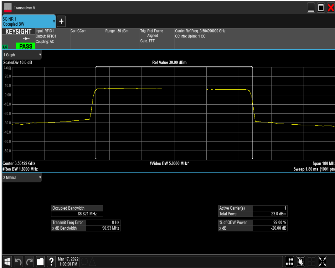
n77(3450-3550) SCS=30kHz DFT_QAM64 BW=90MHz Channel=633666 RB=240@0
