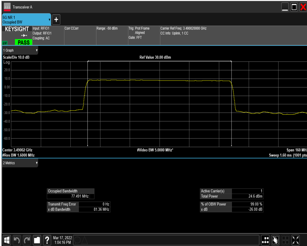
n77(3450-3550) SCS=30kHz DFT_QPSK BW=80MHz Channel=632668 RB=216@0
