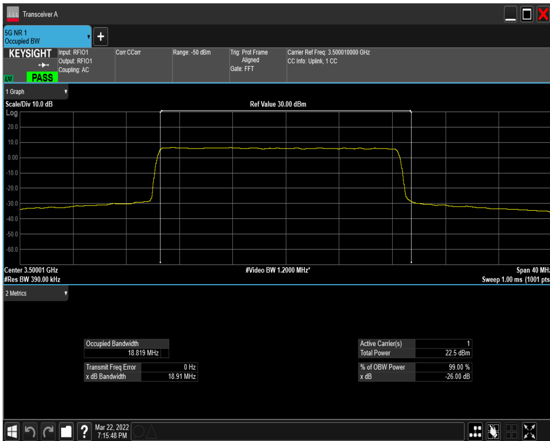
n77(3450-3550) SCS=15kHz DFT_QAM256 BW=20MHz Channel=633334 RB=100@0
