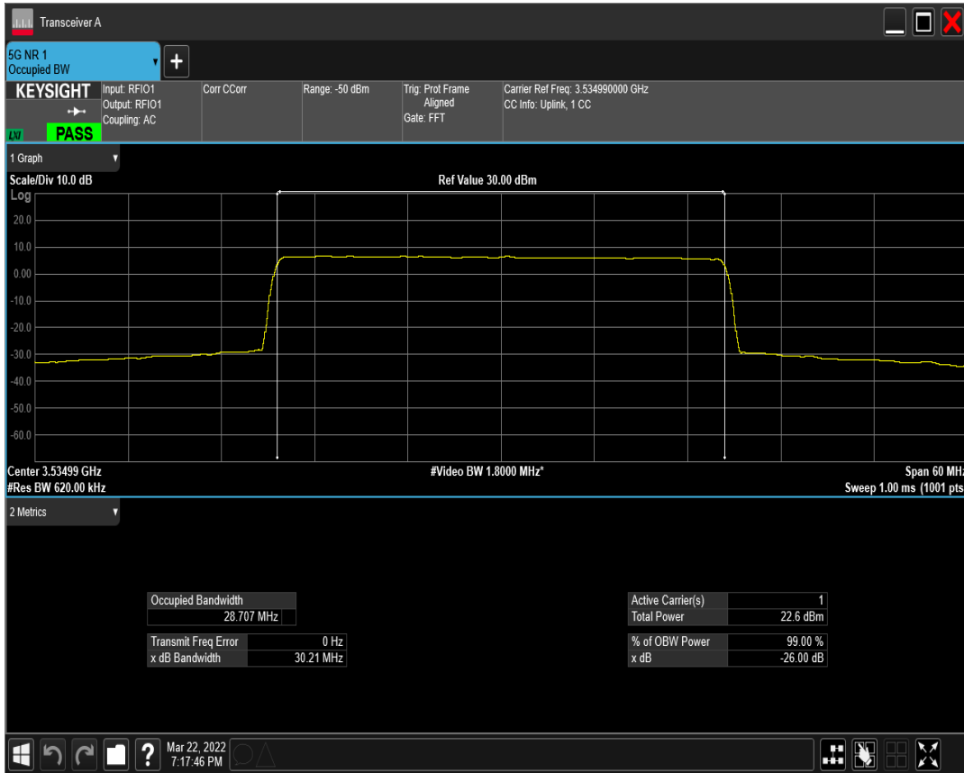
n77(3450-3550) SCS=15kHz DFT_QAM64 BW=30MHz Channel=635666 RB=160@0
