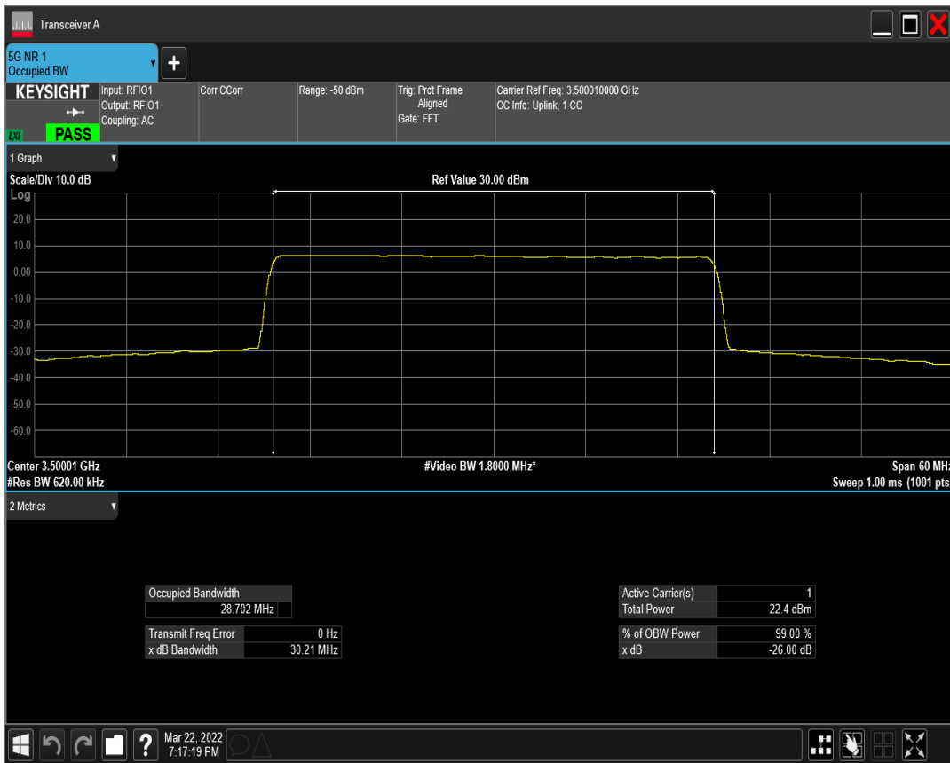
n77(3450-3550) SCS=15kHz DFT_QAM256 BW=30MHz Channel=633334 RB=160@0
