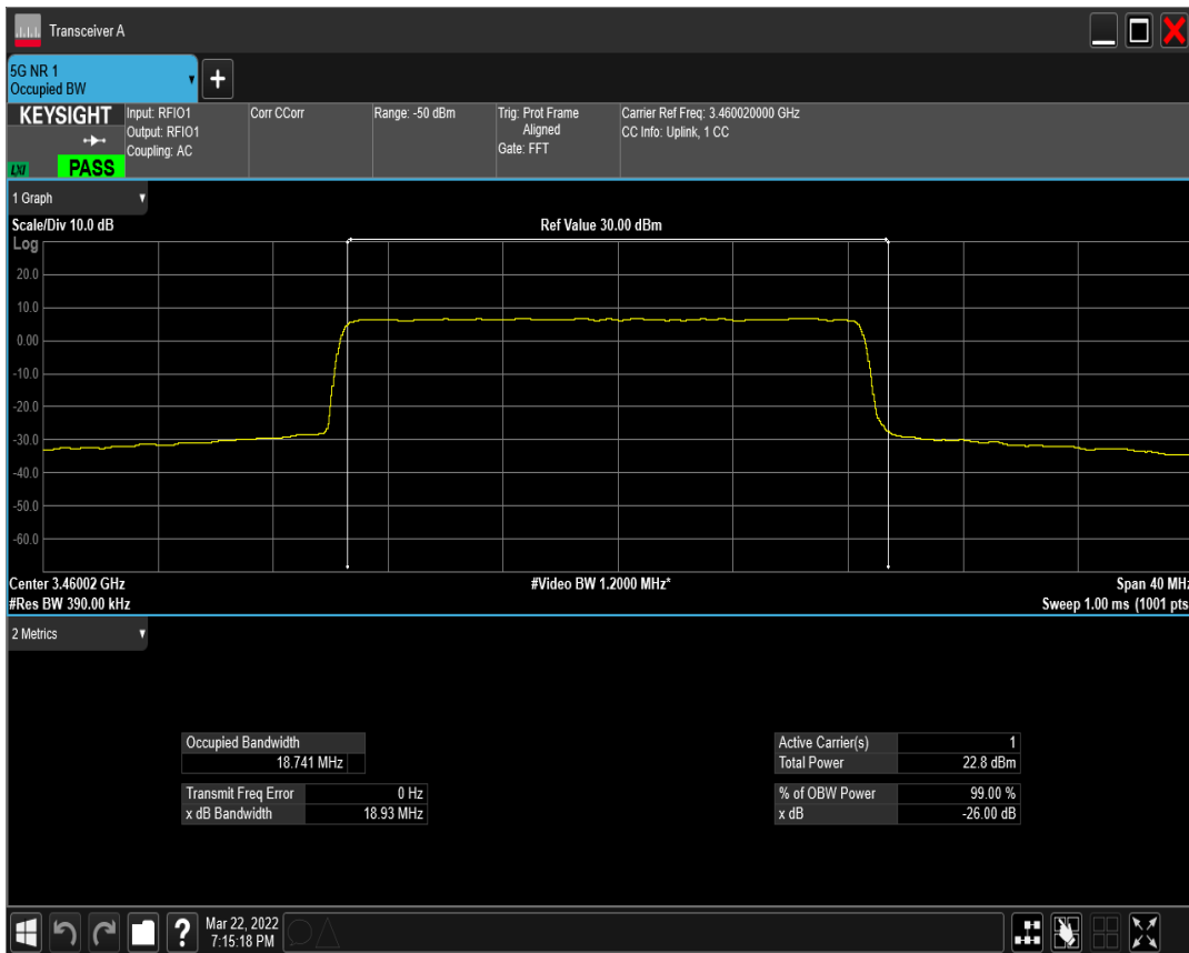
n77(3450-3550) SCS=15kHz DFT_QAM256 BW=20MHz Channel=630668 RB=100@0
