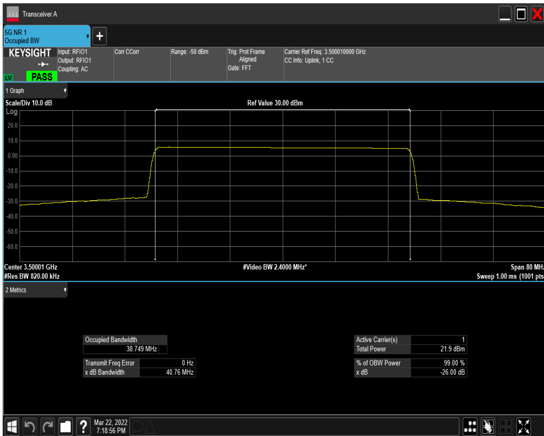
n77(3450-3550) SCS=15kHz DFT_BPSK BW=40MHz Channel=635332 RB=216@0
