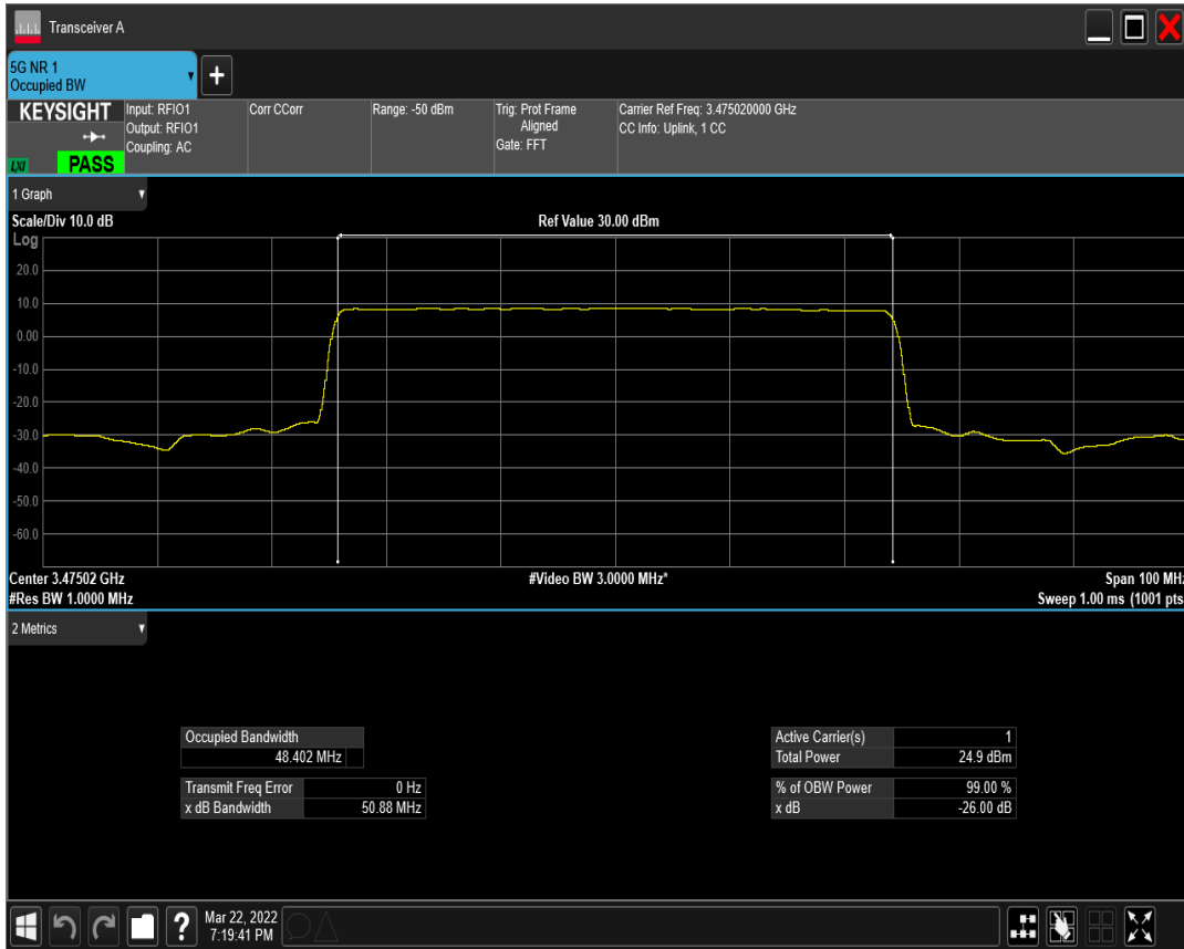
n77(3450-3550) SCS=15kHz DFT_QPSK BW=50MHz Channel=631668 RB=270@0
