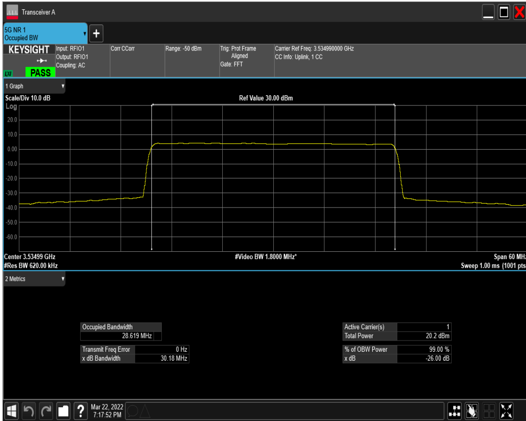
n77(3450-3550) SCS=15kHz CP_QPSK BW=30MHz Channel=635666 RB=160@0
