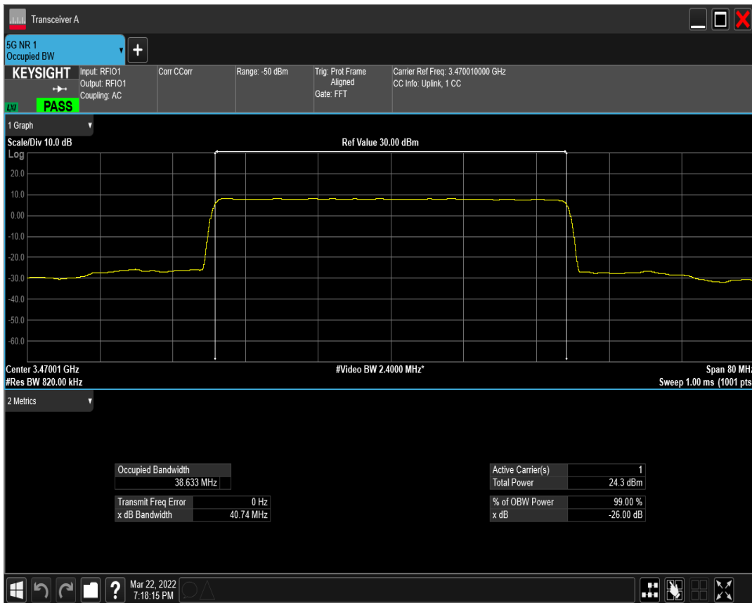
n77(3450-3550) SCS=15kHz DFT_QAM16 BW=40MHz Channel=631334 RB=216@0
