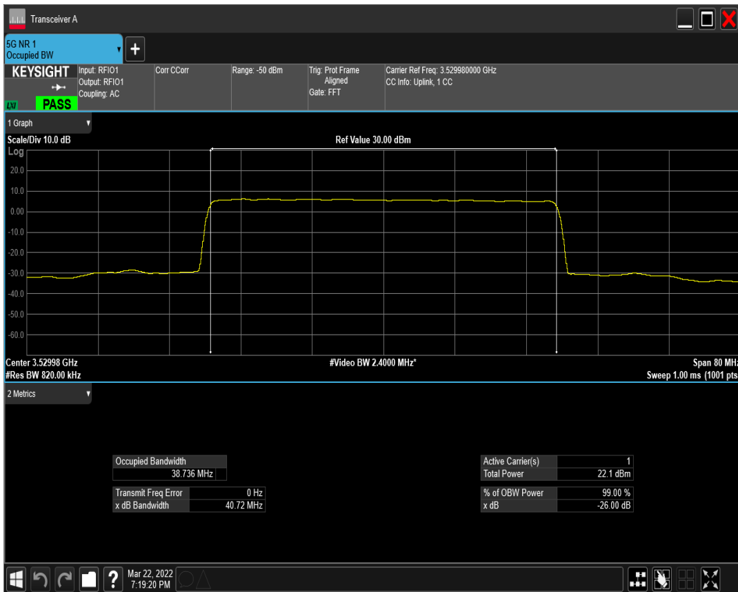
n77(3450-3550) SCS=15kHz DFT_QAM256 BW=40MHz Channel=635332 RB=216@0
