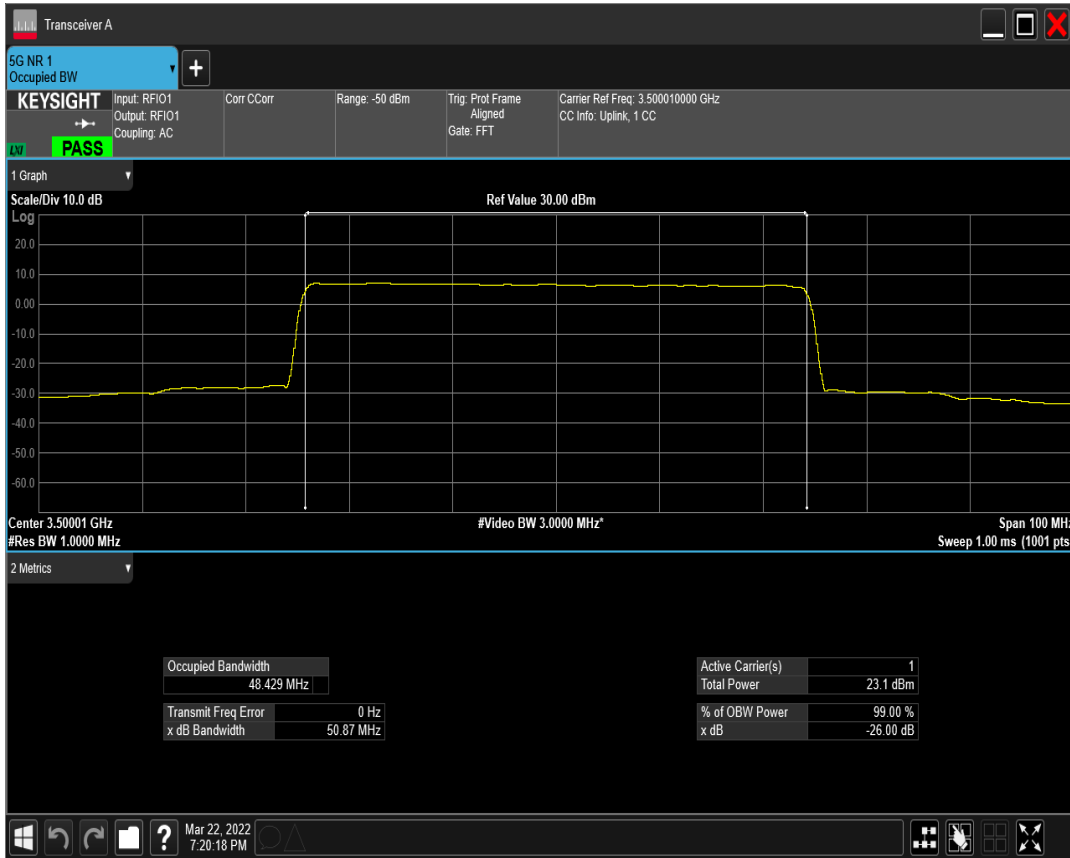
n77(3450-3550) SCS=15kHz DFT_QAM64 BW=50MHz Channel=633334 RB=270@0
