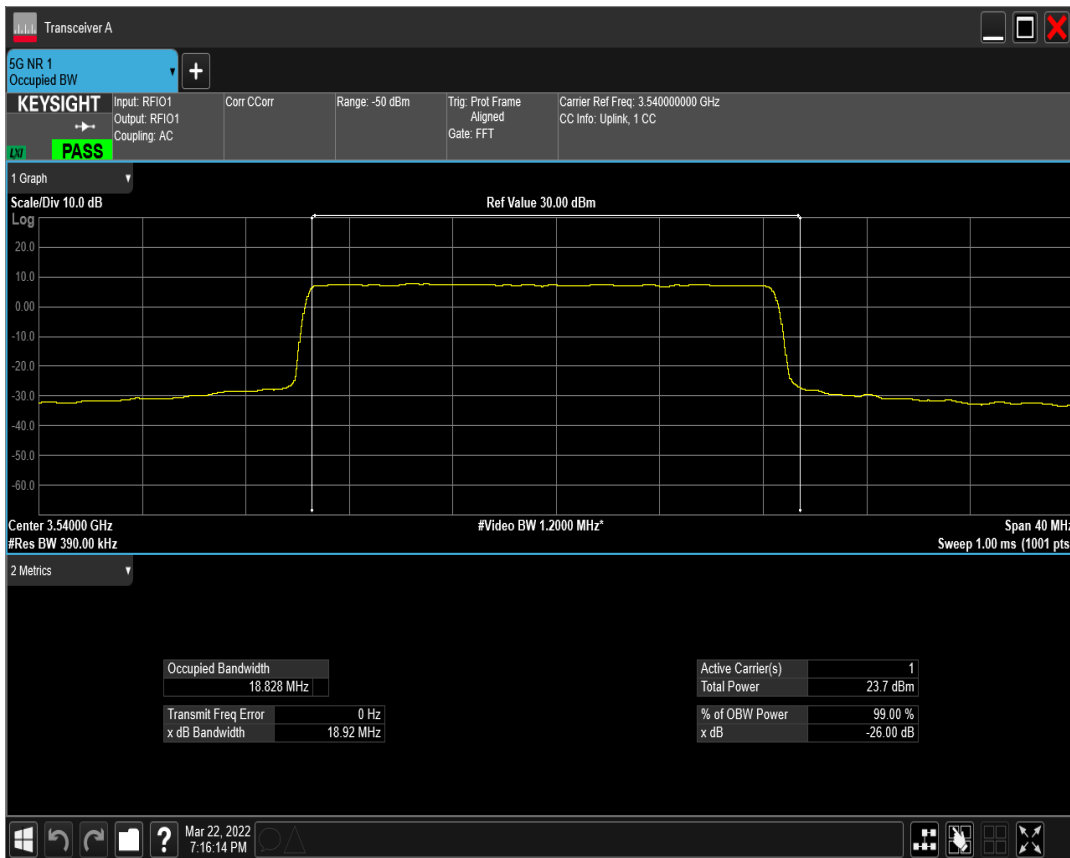
n77(3450-3550) SCS=15kHz DFT_QAM16 BW=20MHz Channel=636000 RB=100@0
