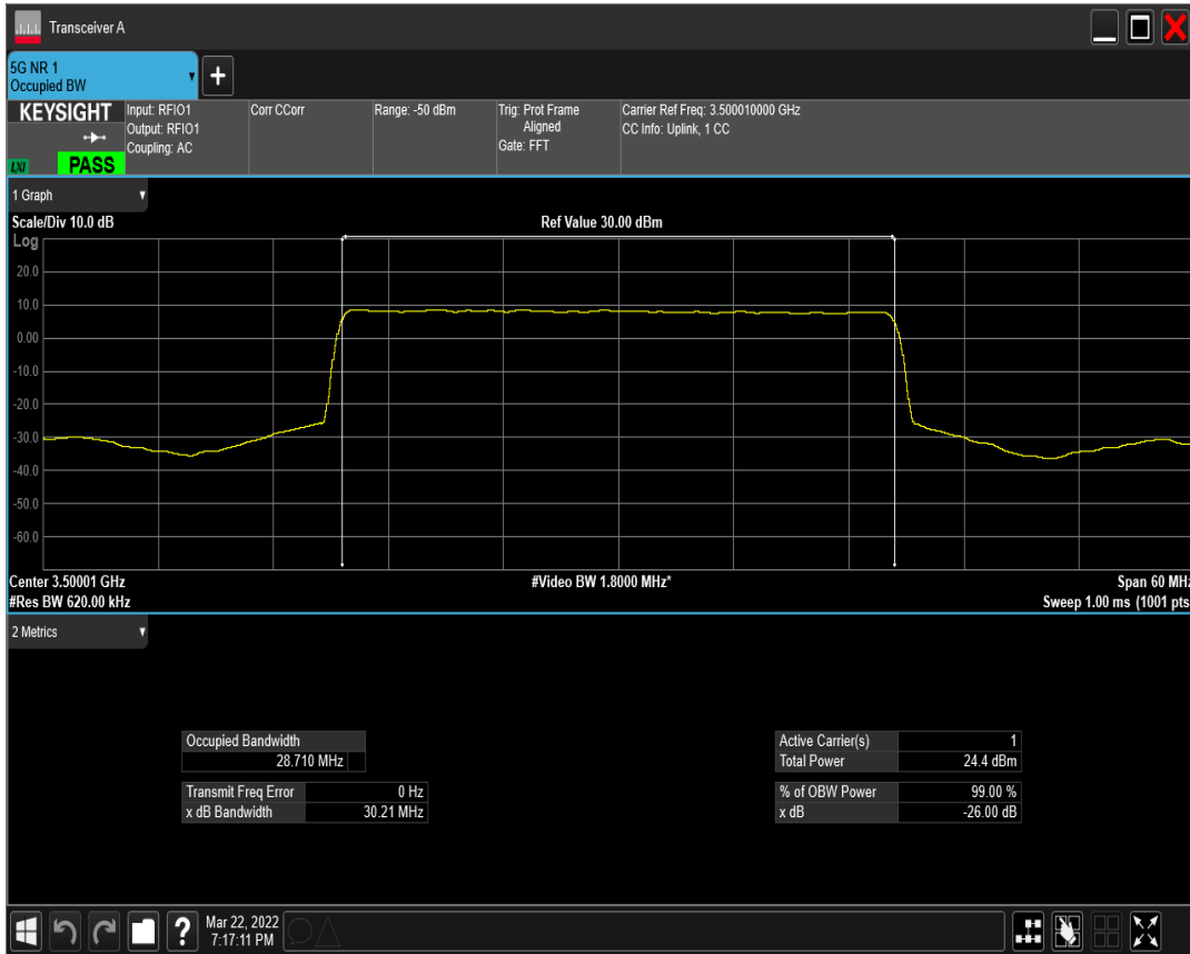
n77(3450-3550) SCS=15kHz DFT_QPSK BW=30MHz Channel=633334 RB=160@0
