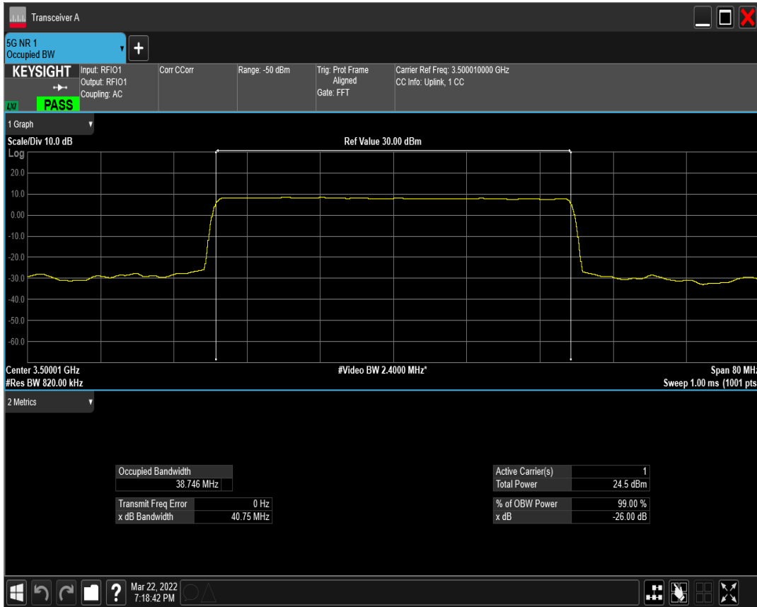
n77(3450-3550) SCS=15kHz DFT_QPSK BW=40MHz Channel=633334 RB=216@0
