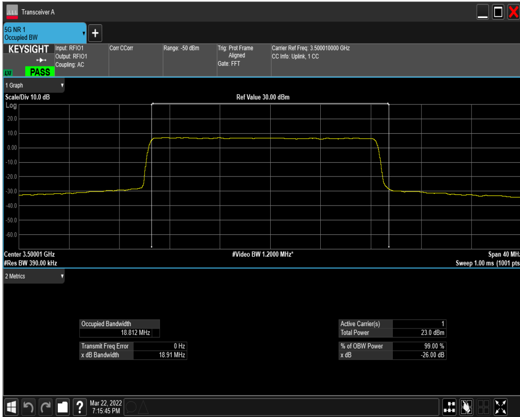
n77(3450-3550) SCS=15kHz DFT_QAM64 BW=20MHz Channel=633334 RB=100@0
