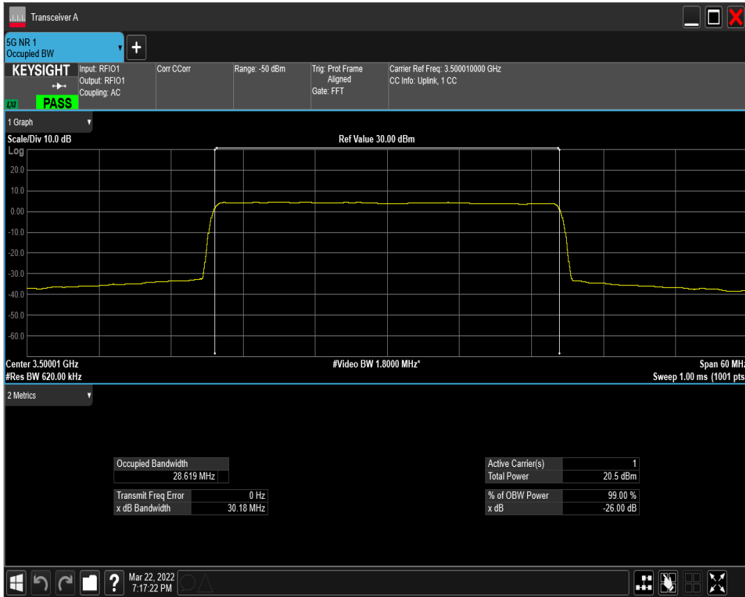
n77(3450-3550) SCS=15kHz CP_QPSK BW=30MHz Channel=633334 RB=160@0
