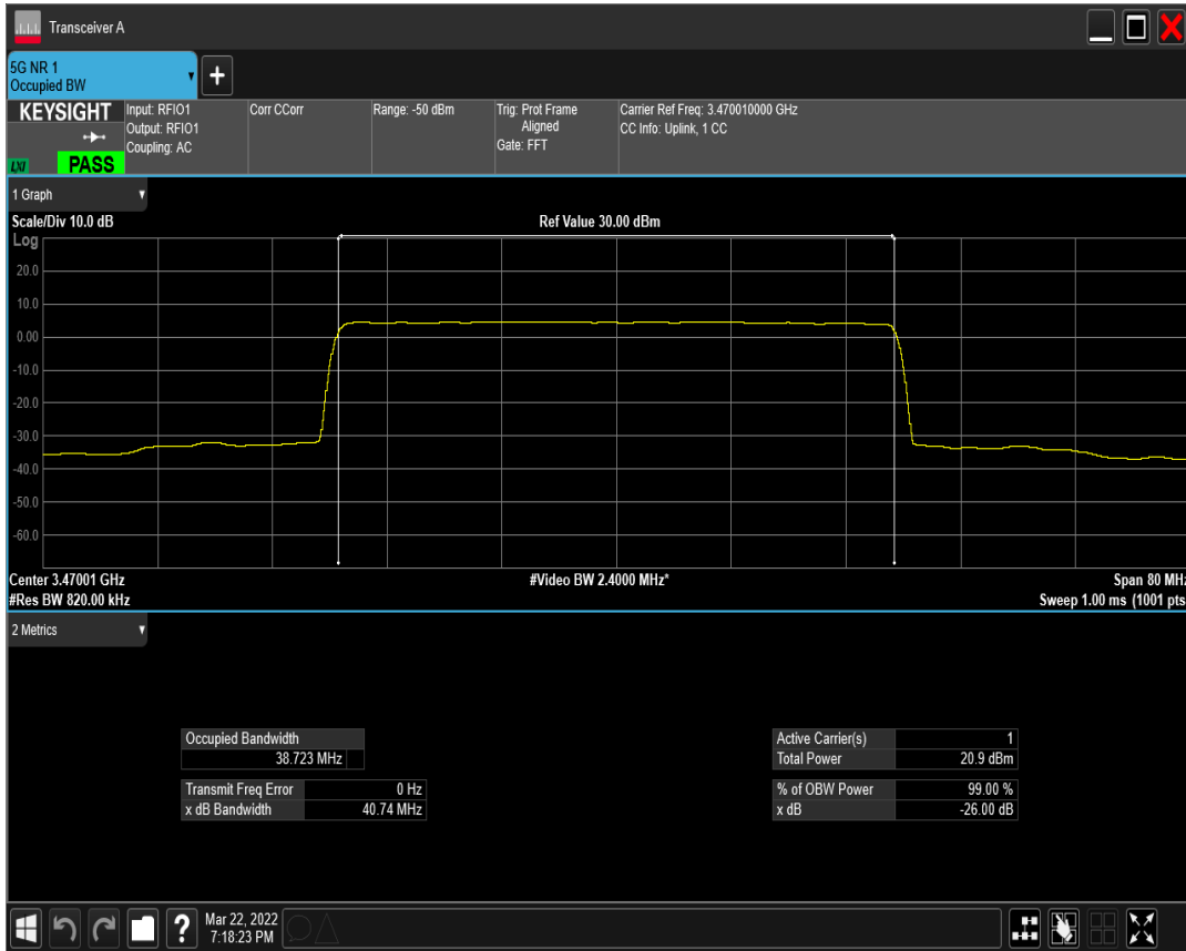
n77(3450-3550) SCS=15kHz CP_QPSK BW=40MHz Channel=631334 RB=216@0
