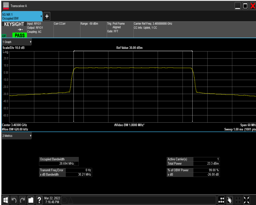
n77(3450-3550) SCS=15kHz DFT_QAM64 BW=30MHz Channel=631000 RB=160@0
