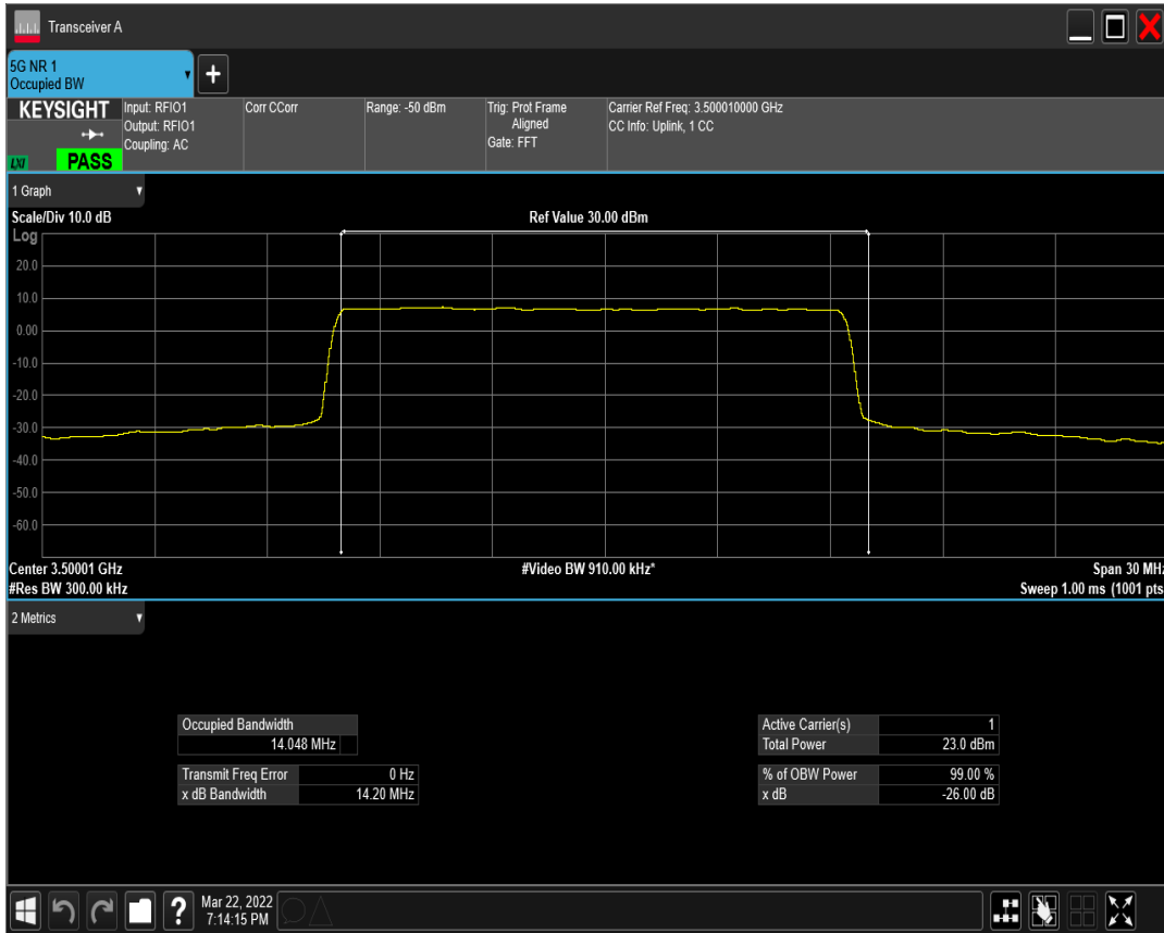
n77(3450-3550) SCS=15kHz DFT_QAM64 BW=15MHz Channel=633334 RB=75@0
