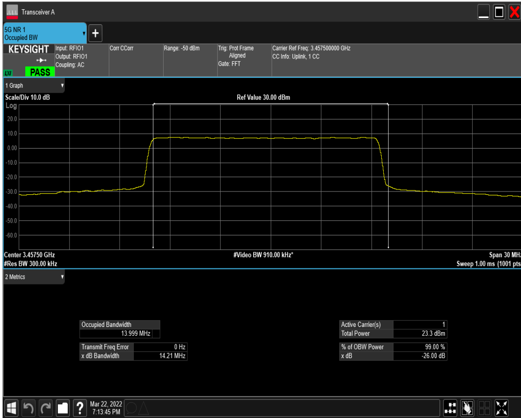
n77(3450-3550) SCS=15kHz DFT_QAM64 BW=15MHz Channel=630500 RB=75@0
