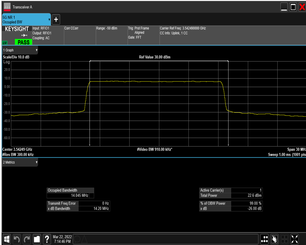
n77(3450-3550) SCS=15kHz DFT_QAM64 BW=15MHz Channel=636166 RB=75@0
