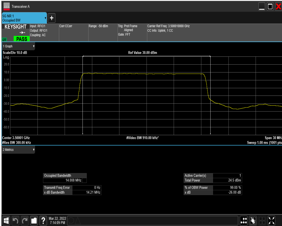
n77(3450-3550) SCS=15kHz DFT_QPSK BW=15MHz Channel=633334 RB=75@0
