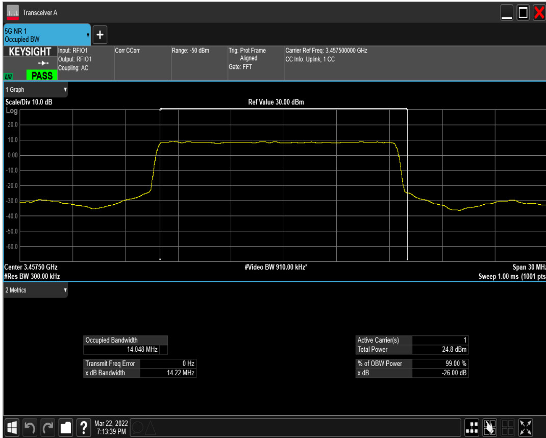
n77(3450-3550) SCS=15kHz DFT_QPSK BW=15MHz Channel=630500 RB=75@0
