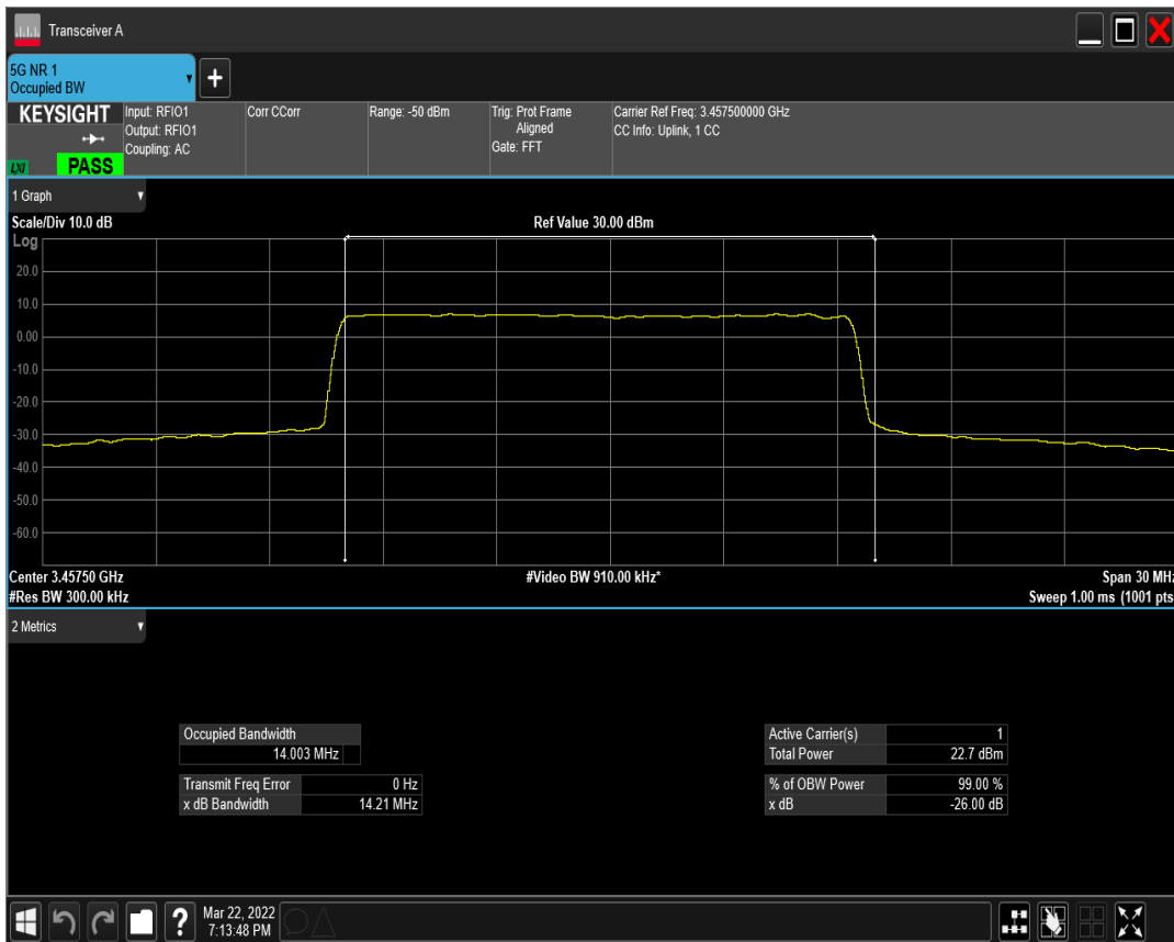
n77(3450-3550) SCS=15kHz DFT_QAM256 BW=15MHz Channel=630500 RB=75@0
