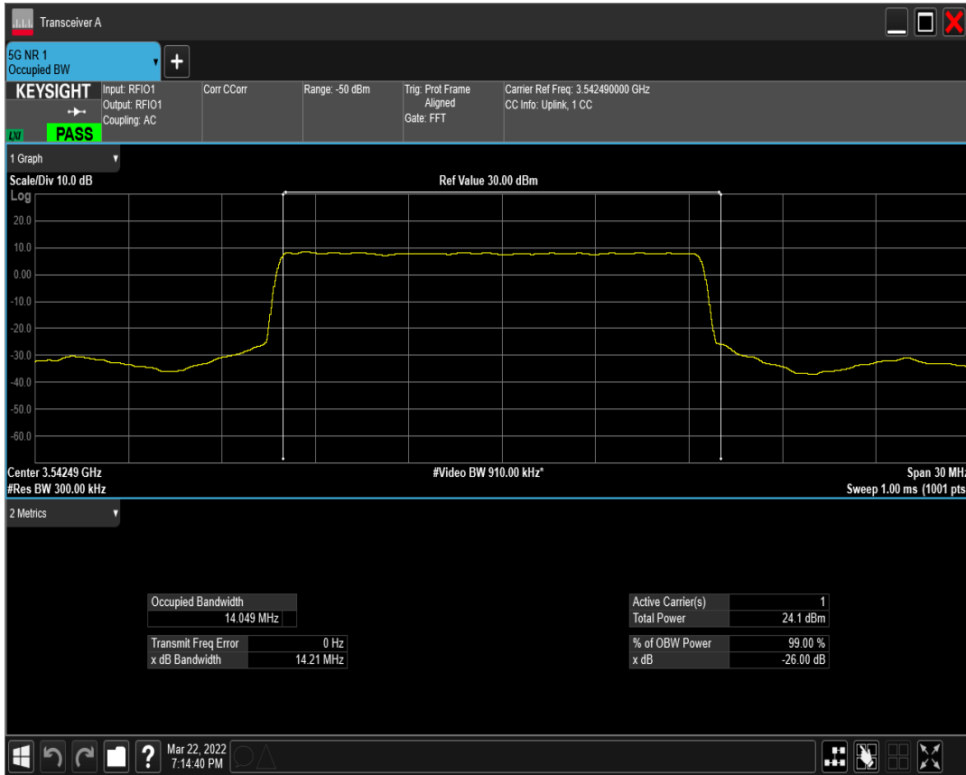
n77(3450-3550) SCS=15kHz DFT_QPSK BW=15MHz Channel=636166 RB=75@0
