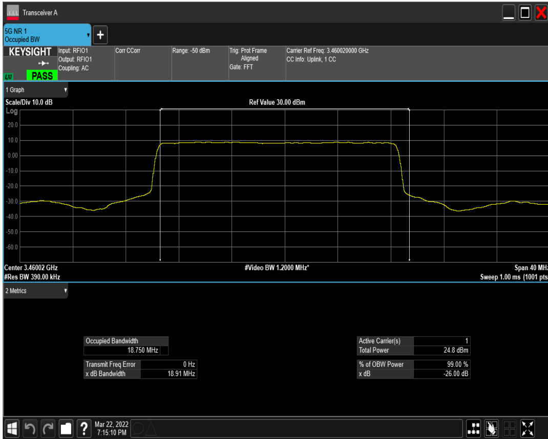
n77(3450-3550) SCS=15kHz DFT_QPSK BW=20MHz Channel=630668 RB=100@0
