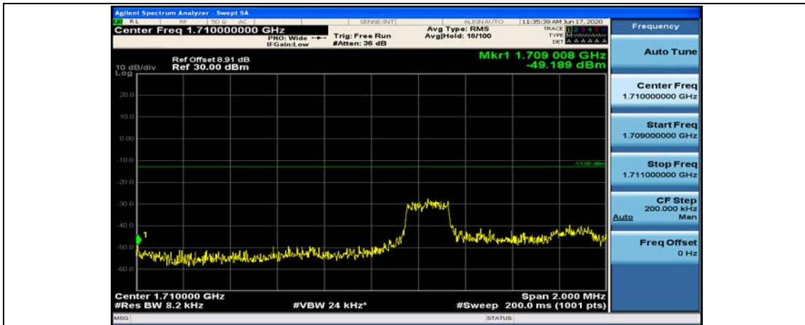
(Channel Bandwidth: 3 MHz)_LCH_QPSK_8RB#0
