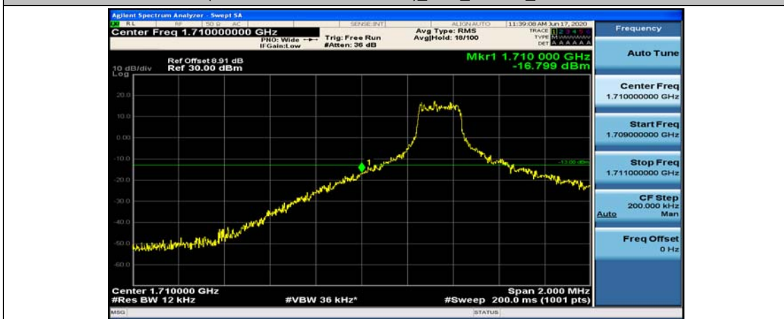
(Channel Bandwidth: 5 MHz)_LCH_16QAM_1RB#12
