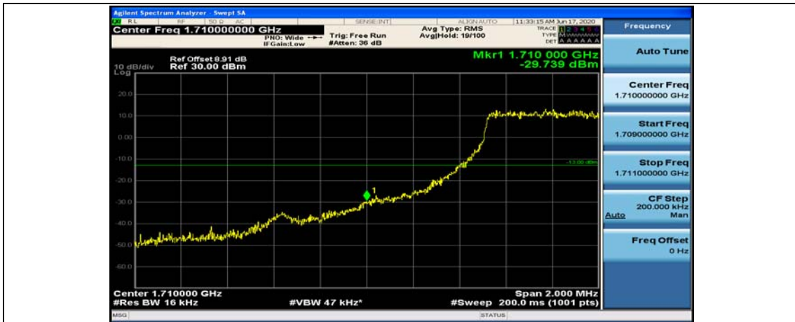
(Channel Bandwidth: 1.4 MHz)_LCH_16QAM_3RB#3
