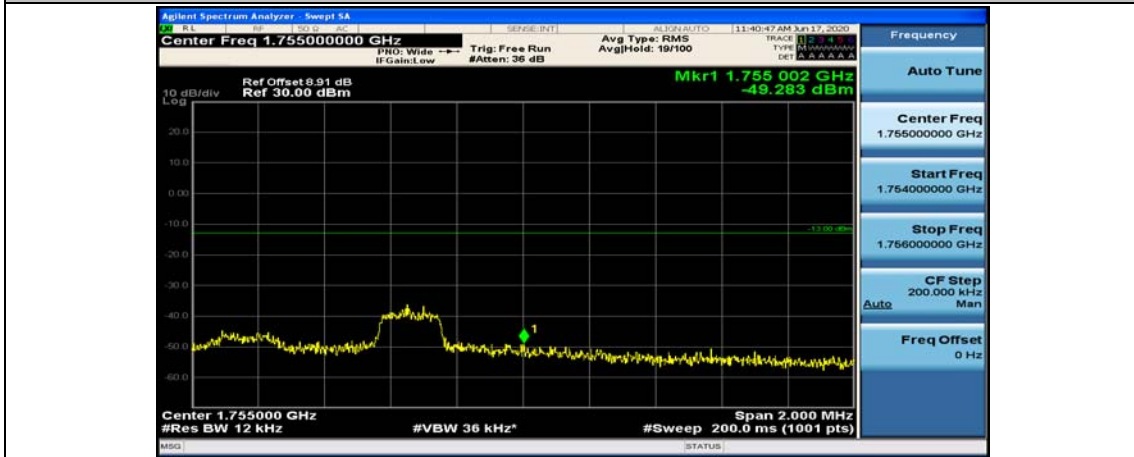
(Channel Bandwidth: 5 MHz)_HCH_16QAM_1RB#12
