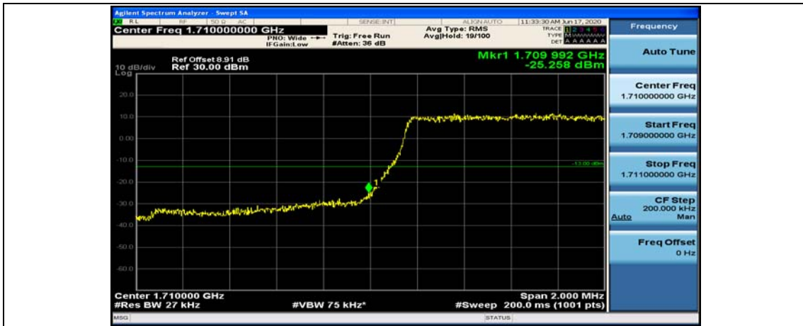
(Channel Bandwidth: 1.4 MHz)_HCH_QPSK_1RB#0
