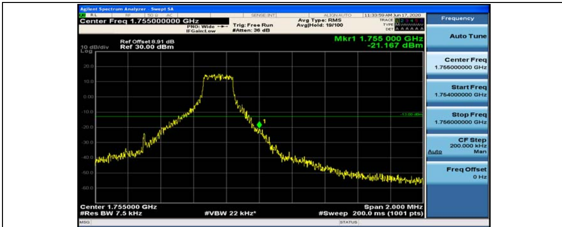
(Channel Bandwidth: 1.4 MHz)_HCH_QPSK_3RB#0
