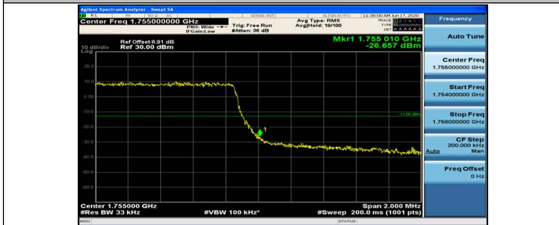
(Channel Bandwidth: 3 MHz)_HCH_QPSK_15RB#0
