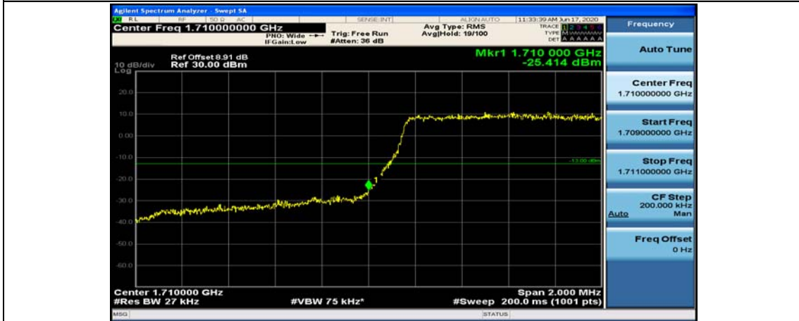
(Channel Bandwidth: 1.4 MHz)_LCH_16QAM_6RB#0
