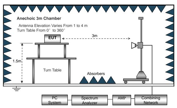
Frequency:30MHz-1GHz Frequency:9kHz-30MHz Frequency: Above 1GHz RBW=10KHz. RBW=120KHz. RBW=1MHz, VBW = 30KHzVBW=300KHz VBW=3MHz(Peak), 10Hz(AV) Sweep time= Auto Sweep time= Auto Sweep time= Auto Trace = max holdTrace = max holdTrace = max holdDetector function = peak Detector function = peak, QP Detector function = peak, AV
