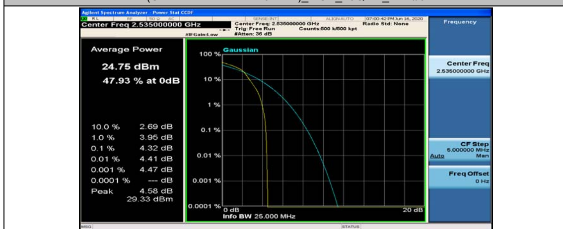
(Channel Bandwidth:20 MHz)_MCH_16QAM_1RB#49
