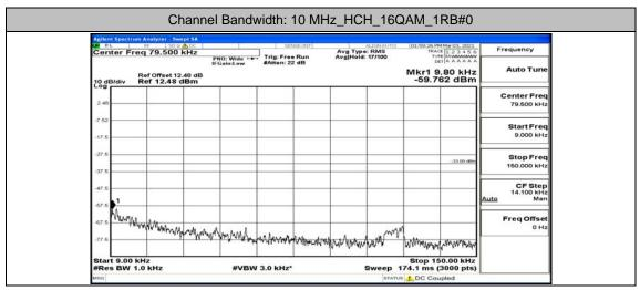
Stop Freq 150.000 kHz CF Step 14.100 kHz
