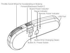
**Power on/off:** Long press the button "A" for power on; long press the button "A" again for power off.
