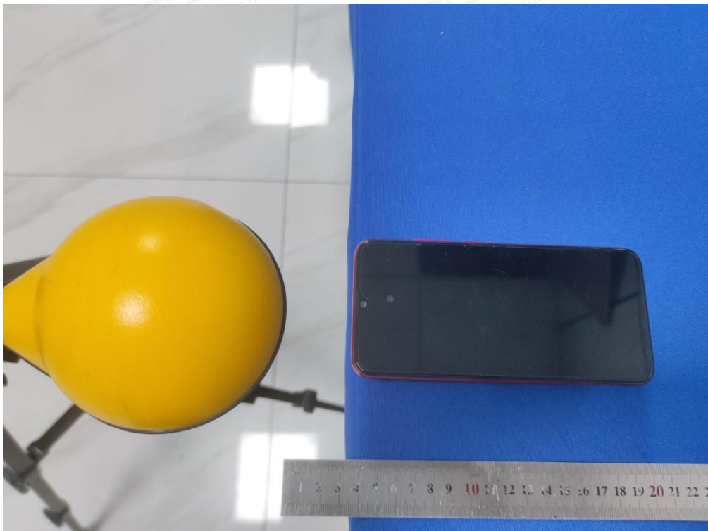
Test Position D(4cm) - Exposure photo from side edge surface-Front(TM1)
