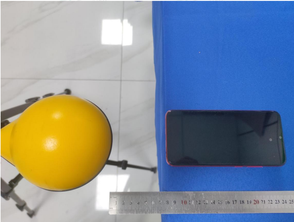
Test Position B(8cm) - Exposure photo from side edge surface-Rear(TM1)
