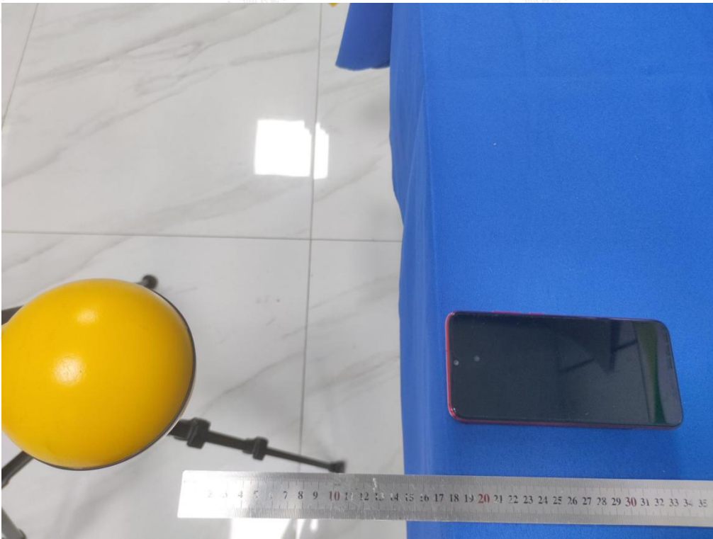
Test Position D(18cm) - Exposure photo from side edge surface-Front(TM1)
