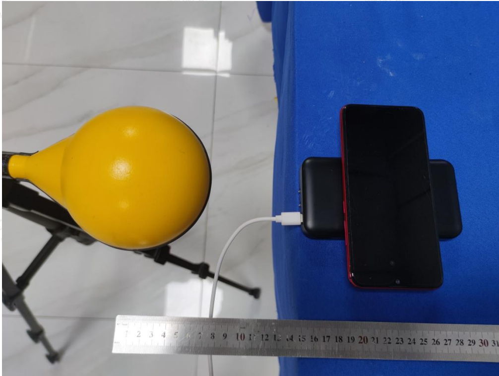
Test Position B(15cm) - Exposure photo from side edge surface-Rear(TM1)
