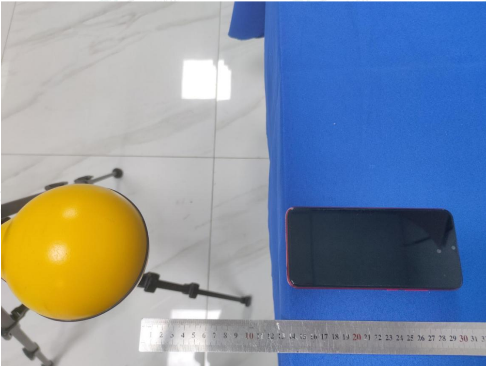
Test Position B(14cm) - Exposure photo from side edge surface-Rear(TM1)
