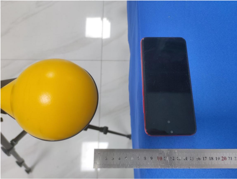
Test Position E(8cm) - Exposure photo from side edge surface-Right(TM1)
