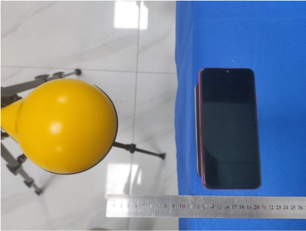
Test Position C(12cm) - Exposure photo from side edge surface-Left(TM1)
