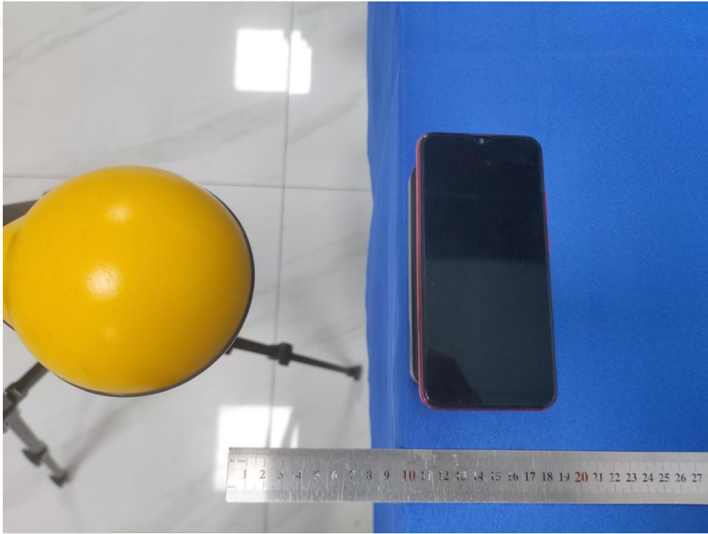
Test Position C(10cm) - Exposure photo from side edge surface-Left(TM1)
