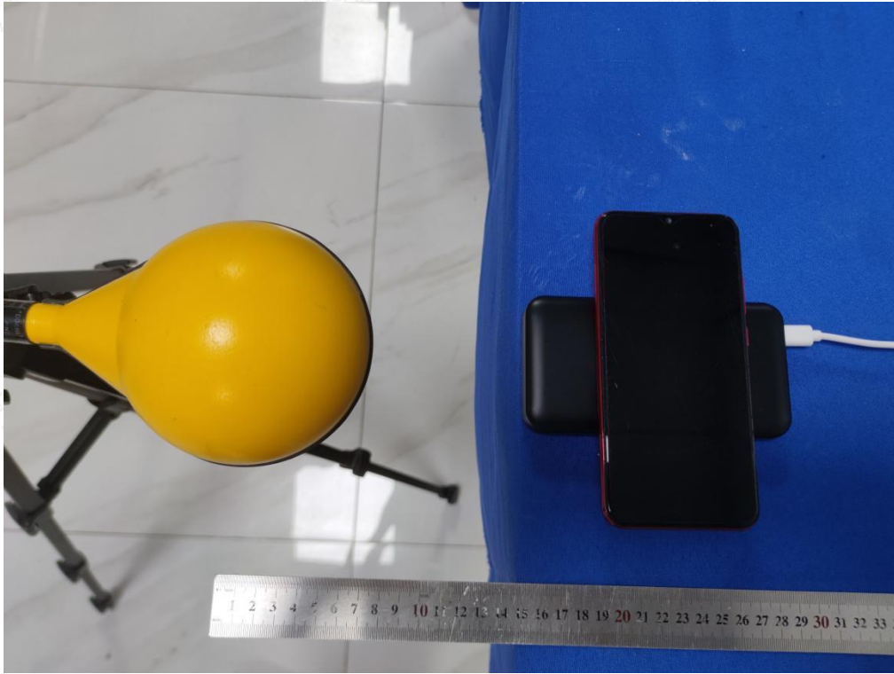
Test Position D(15cm) - Exposure photo from side edge surface-Front(TM1)
