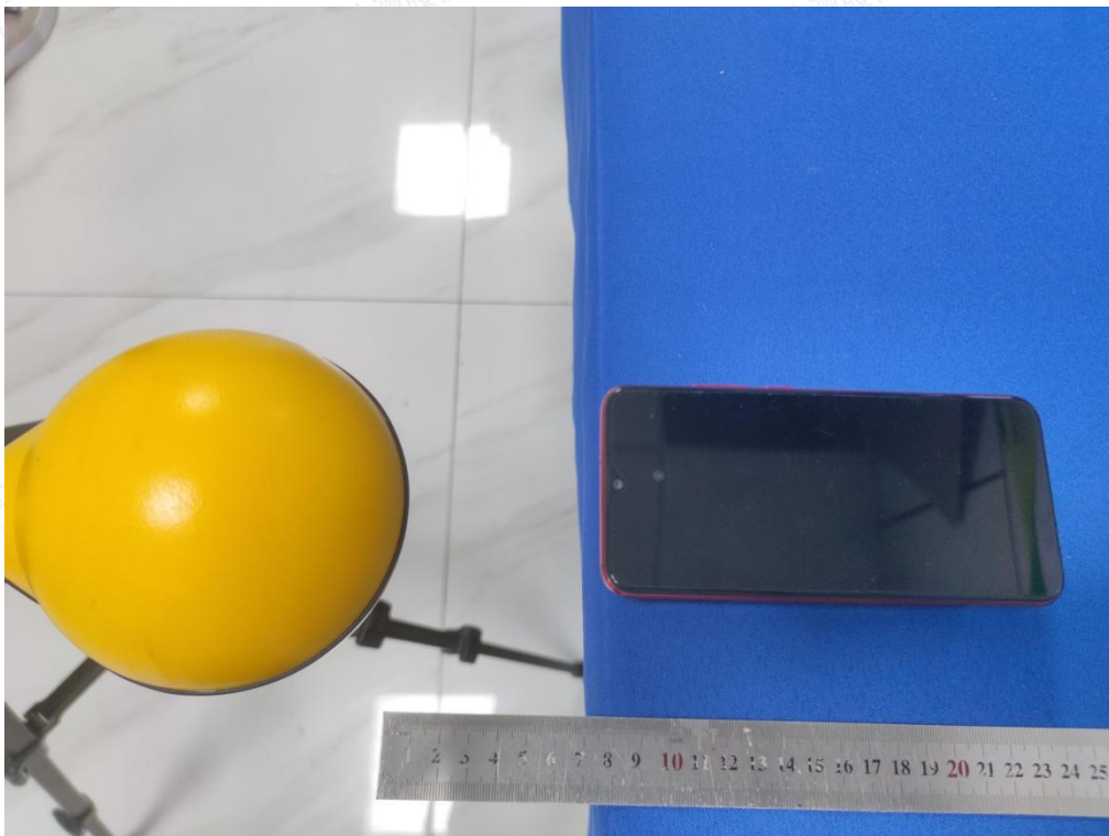
Test Position D(8cm) - Exposure photo from side edge surface-Front(TM1)
