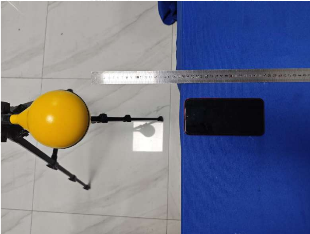
Test Position F(20cm) - Exposure photo from bottom surface(TM1)
