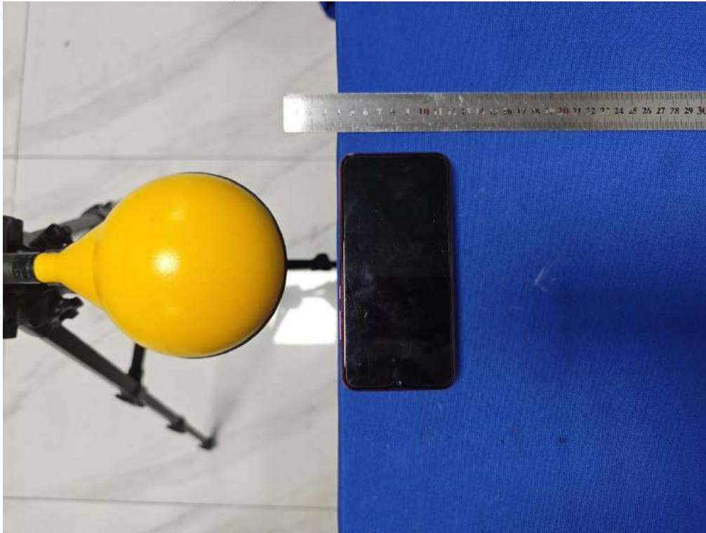
Test Position E(4cm) - Exposure photo from side edge surface-Right(TM1)
