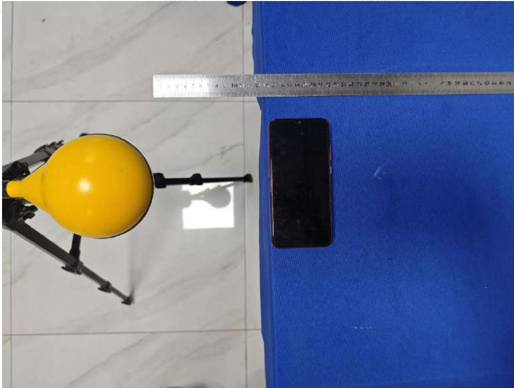
Test Position C(14cm) - Exposure photo from side edge surface-Left(TM1)
