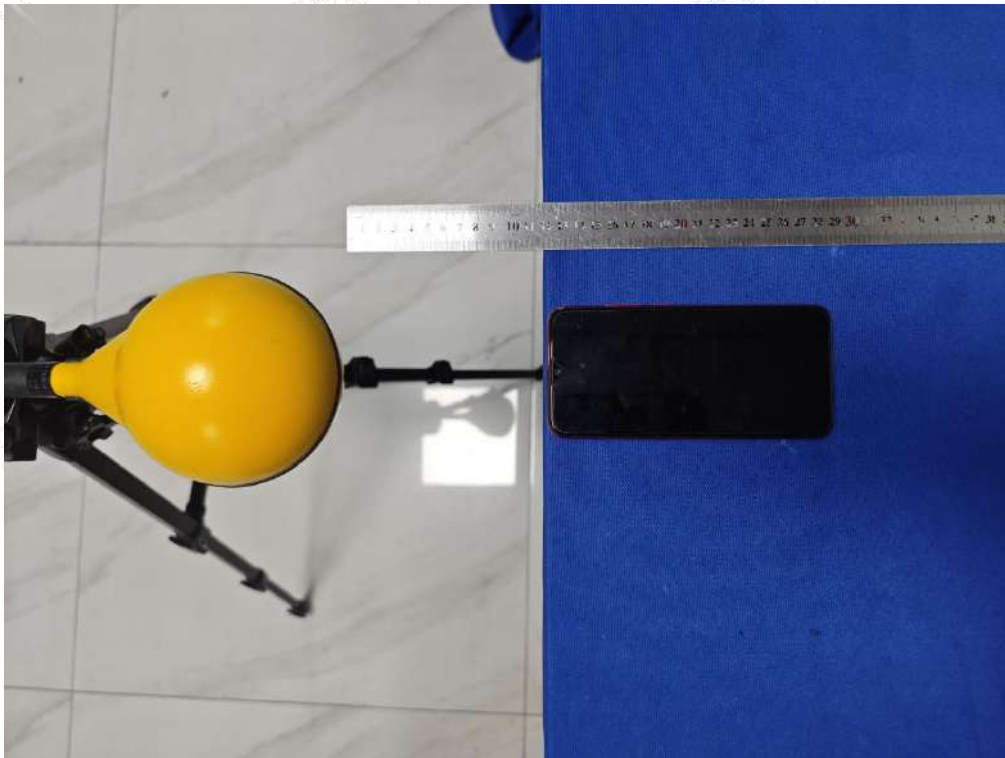
Test Position F(12cm) - Exposure photo from bottom surface(TM1)
