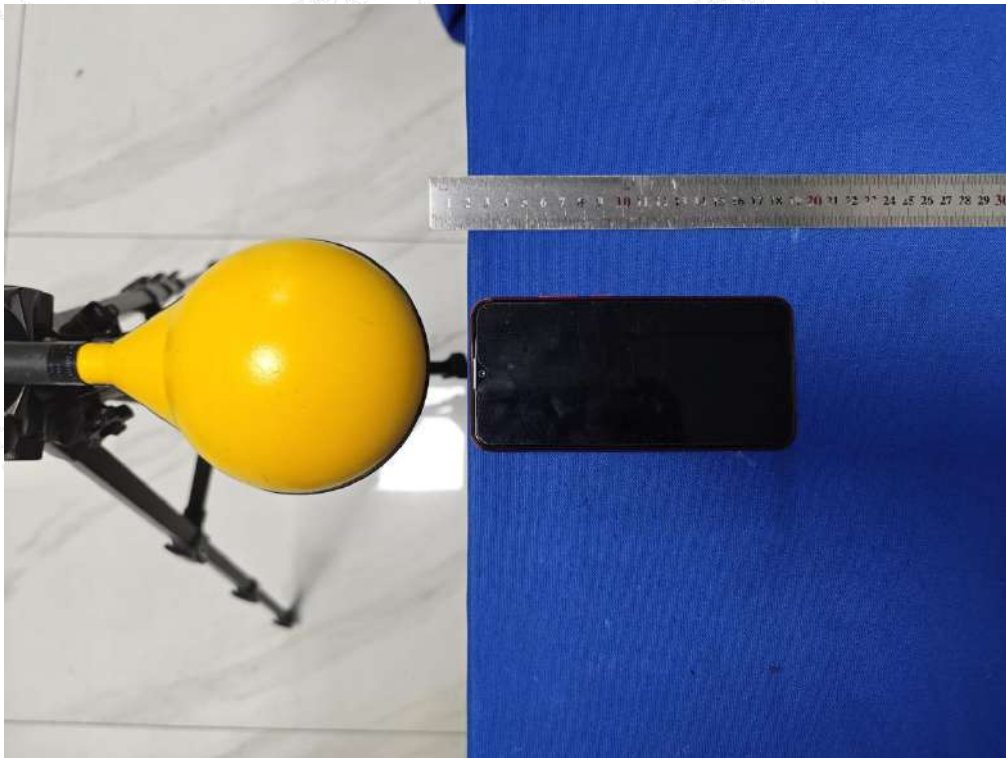
Test Position F(2cm) - Exposure photo from bottom surface(TM1)
