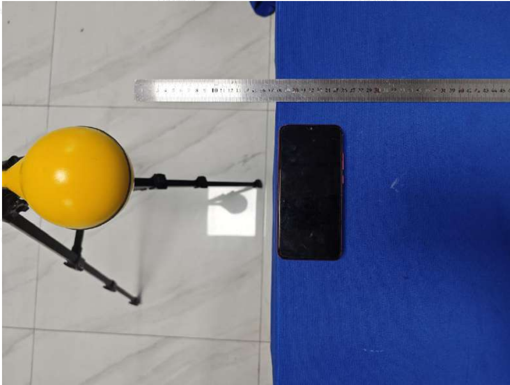
Test Position C(18cm) - Exposure photo from side edge surface-Left(TM1)
