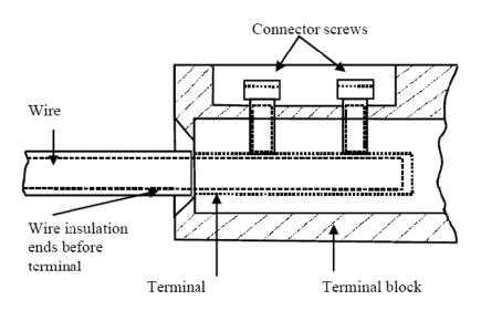
7. The cables should be connected correctly according to the wiring diagram and the terminals should be tightened during the installation in order to avoid any damage caused by bad connection.
