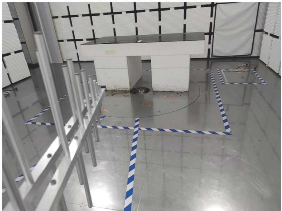
Radiation Emission Test Setup (30MHz to 1GHz)
