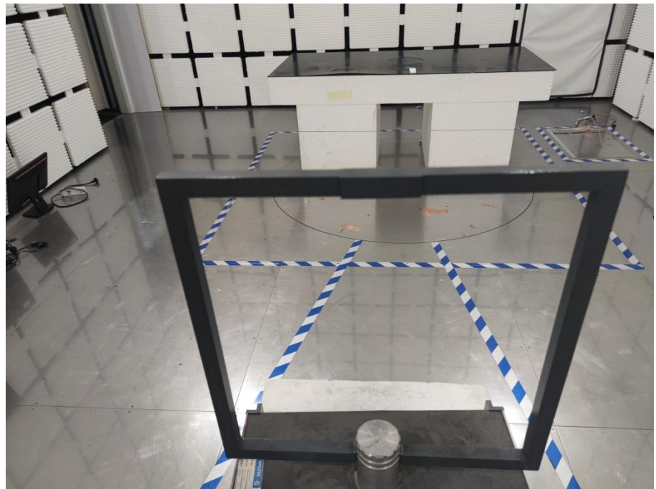
Radiation Emission Test Setup (Below 30MHz)
