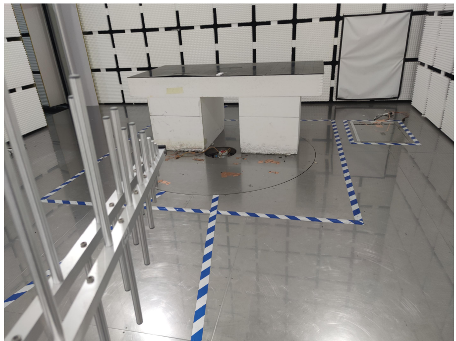
Radiation Emission Test Setup (30MHz to 1GHz)
