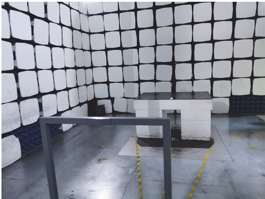
Radiation Emission Test Setup (Below 30MHz)
