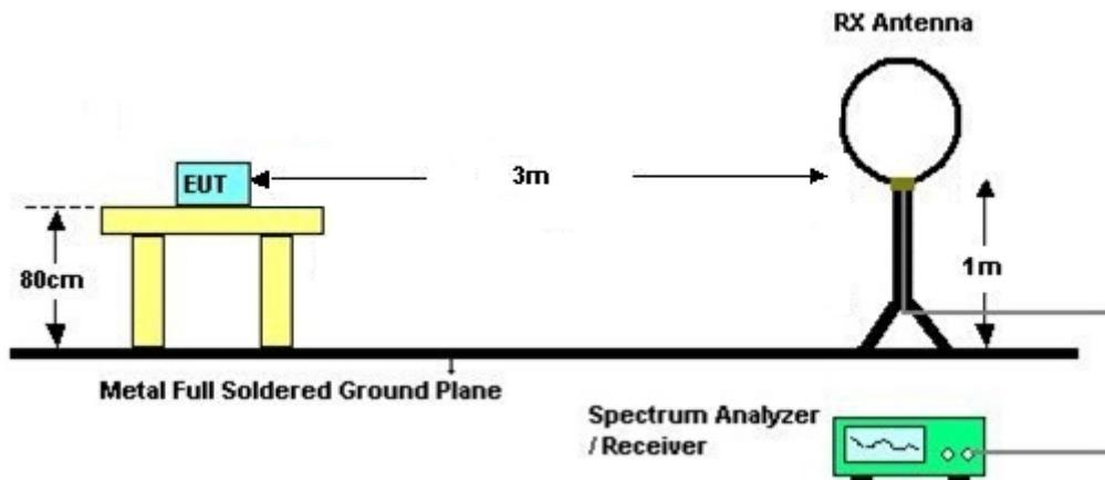
For radiated emissions from 30MHz to 1GHz
