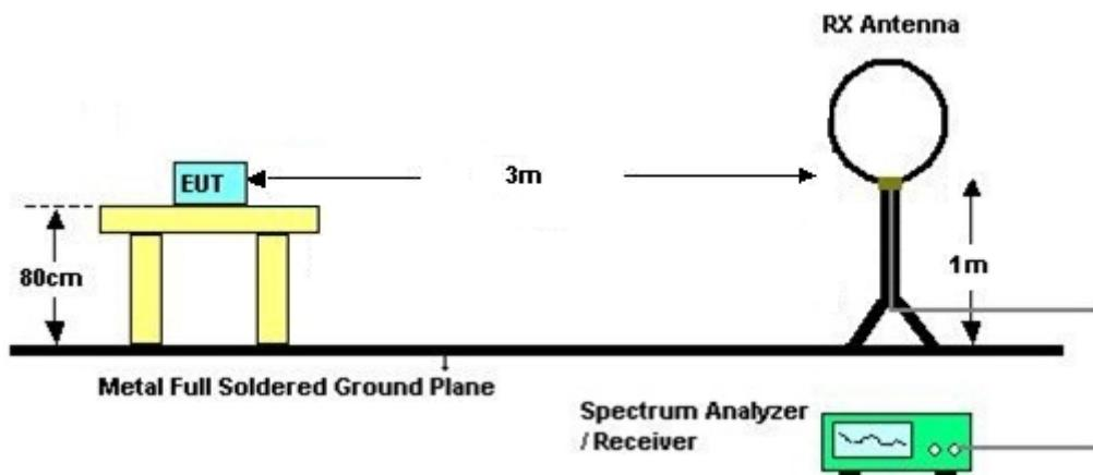
For radiated emissions from 30MHz to 1GHz
