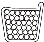
Asymmetrical crimping shape. Burr formation on one side.
