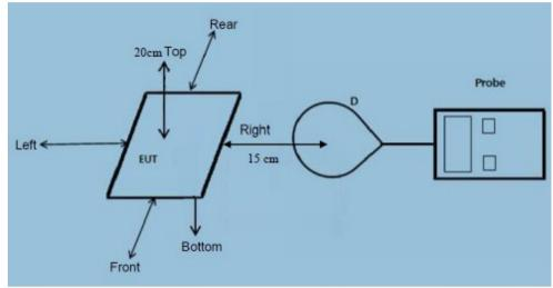
Remark: The E300 probe antenna diameter is less than 11.5cm.
