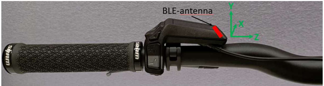
Figure 3.0. BLE-antenna positioning and orientation during to measurements.
