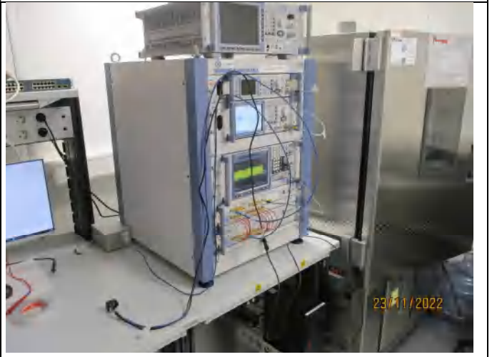
Conducted test set up
