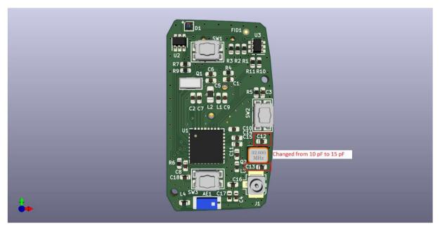
Internal view from right side - The changed capacitors are C12 and C13 in the picture.
