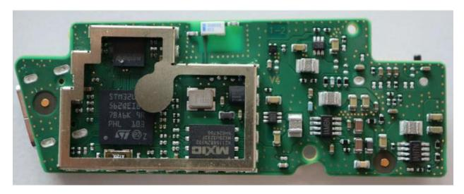
Figure 6, Vertical PCB, Downside, Radio components
