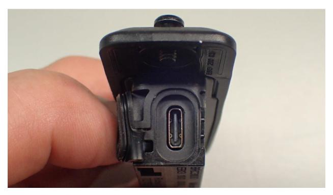
Figure 7, Backside, USB connector cover open
