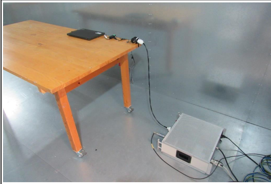
Setup for measurements 150 kHz - 30 MHz
