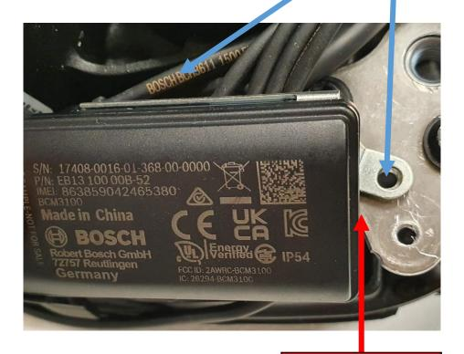
Avoid clamping any cables between CP and BCM.
