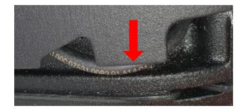
If BCM1 cable is clamped by design cover, push it back underneath before mounting the Design Cover screw.
