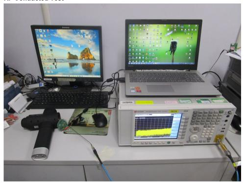
Conducted Emissions at AC Power Line (150kHz-30MHz)
