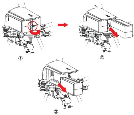
1.4 Installation of remote controller antenna
