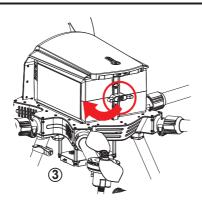
Note: If the battery or its lock is not fastened normally, it may lead to poor contact of power supply, affect the flying safety, even flying failure and affect the flying experience.
