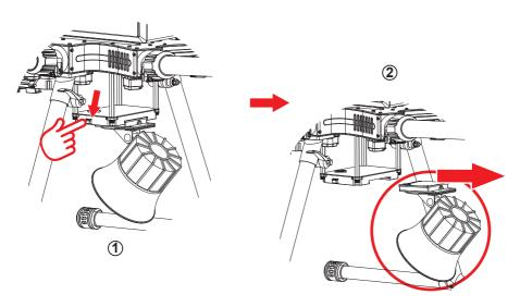
Removal of double payload mounts. As shown in figure below:
