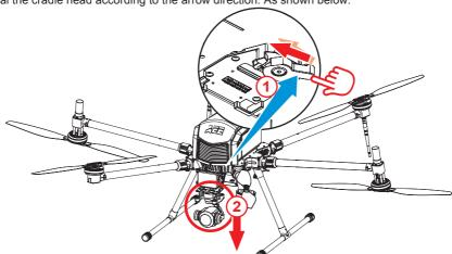
While removal the cradle head, hold the cradle head with one hand and removal it with another hand, to avoid falling and damage of cradle head.
