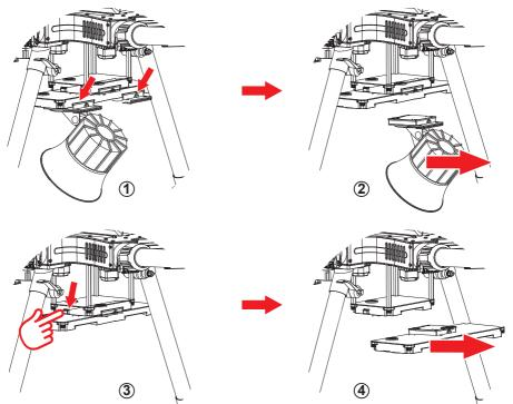
Prompt: While removal the payload mount, hold the unlock button with one hand, hold the payload mount with another hand and move it out slowly according to the direction in diagram, to avoid falling and damage of payload mount during removal.
