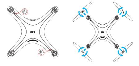
Left hand thread propeller has a mark "P" on the propeller and fastens to motor with a "P" marked on the arm of the drone near the motor. Right hand thread propeller has no marks on the propeller and no marks on the arm of the drone.
