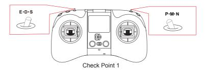
Set Right Hand Toggle Switch In "P" Position (GPS mode).
