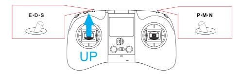
(If you find the drone spin around in circles, lift it up to 30 meters, wait until it hover steady, and then land the drone and do re-calibration).
