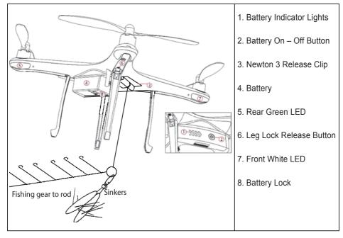
**Note:** The release wire loop connector connects with one wire loop into the Newton 3 release clip and the loop at the other end connects to the weights and 6-hook section with the clip on the end of the hook section. The wire is laid straight in front of the drone prior to take off and keeps the line well away from the propellers during take off and release actions. **Do not use the drone for fishing without the correct release wire!**
