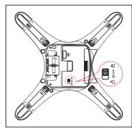
Check Point 2. Insert Battery Correctly
