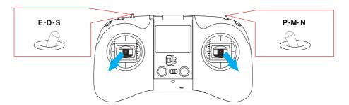
This lever position is also the emergency shutdown so NEVER pull both levers down at 45% outwards when flying as you will crash your drone due to motor shutdown. Use one lever at a time while learning to avoid any issues.
