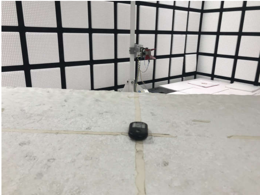
Radiated spurious emission Test Setup-2(Above 1GHz)
