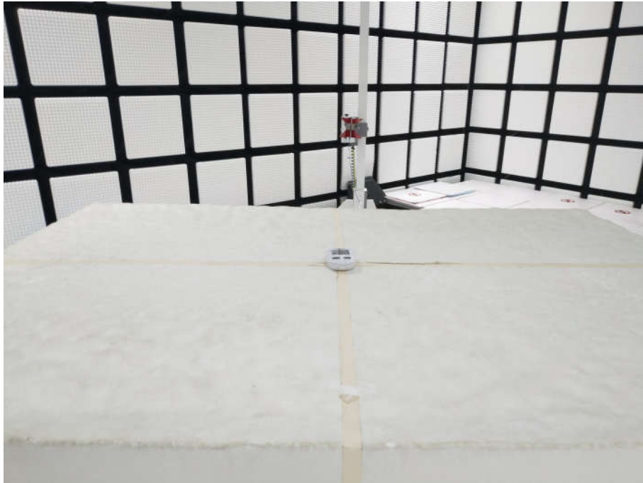
Radiated spurious emission Test Setup-3(Above 1GHz)
