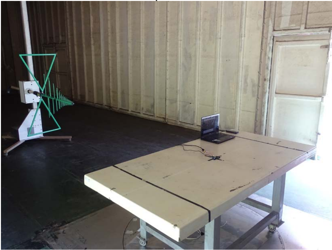
Front View of Spurious Emission Test
