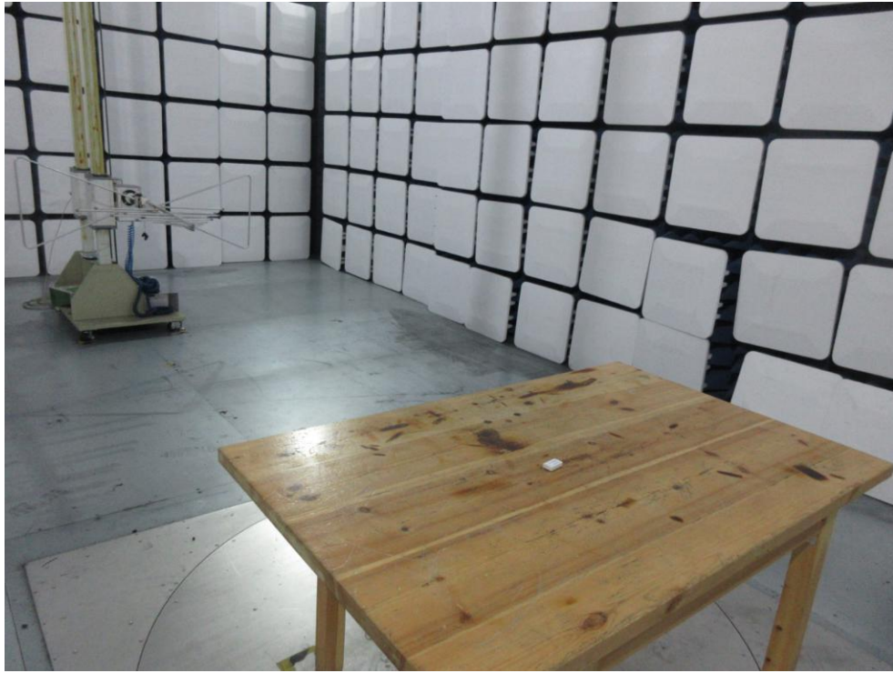
FCC ID: 2AWOQ-GK100 Photo of Radiation Emission Test
