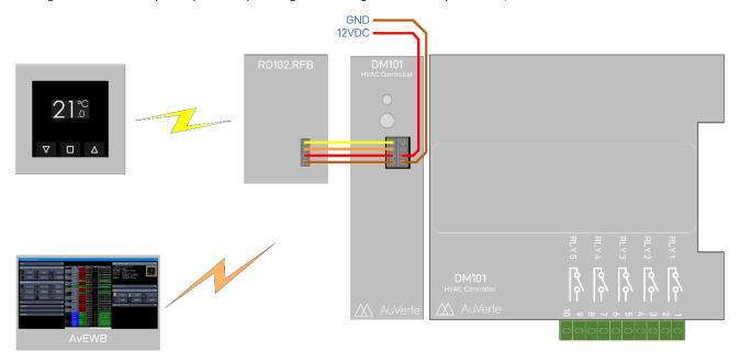
The image to the right shows how a number of daisy chained DM10x controllers use the RD102RFB device to provide communication capabilities when fully enclosed in a sheet metal housing.
