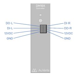
The figure below shows an example how the front-side I/Os can be used. The left digital output (DO-L) is used to drive a relay with a 12VDC coil. DO-L and DO-R both feature a free-run diode to avoid damaging the output when the relay is turned off. The right digital output (DO-R) is driving directly an LED. Both outputs feature a current setting capability that run 1mA through the pushed output. This avoids that the LED will require an external current limiting resistor.
