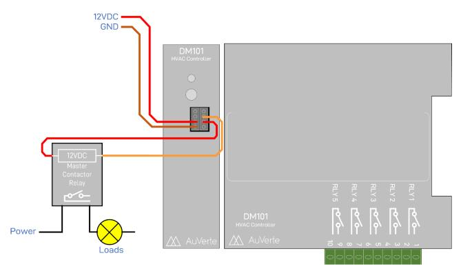
As an example, the chassis-mount T9AP1D52-12 by TE Connectivity Potter & Brumfield Relays can be used for such an application. The designer of such a deployment needs to assure that all local electrical code requirements have been met.
