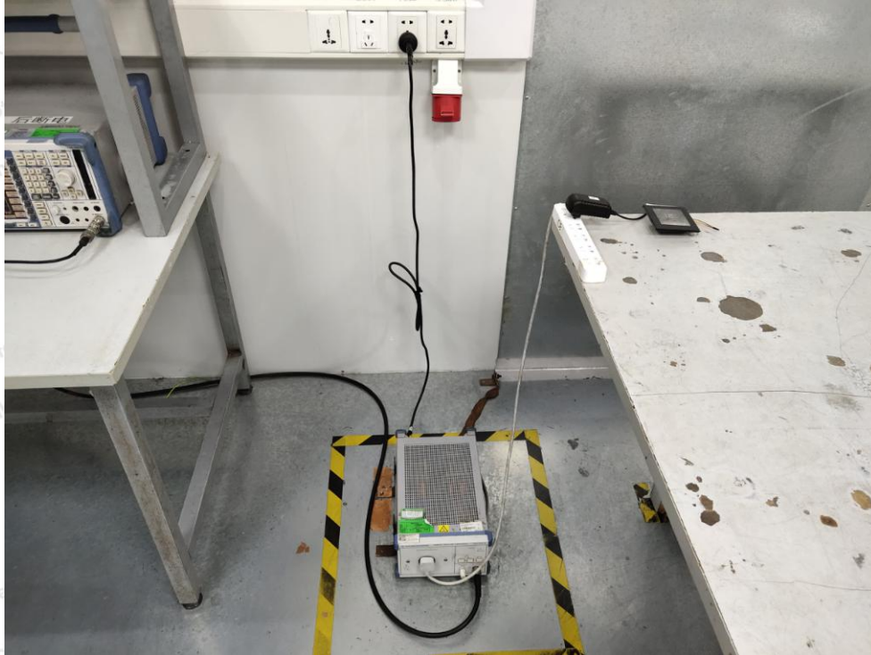
Photo of Power Line Conducted Emission Test
