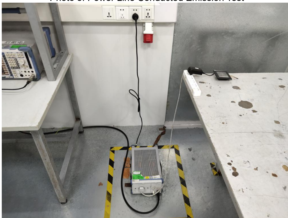
FCC ID: : 2AWOQ-003001C508 Photo of Power Line Conducted Emission Test
