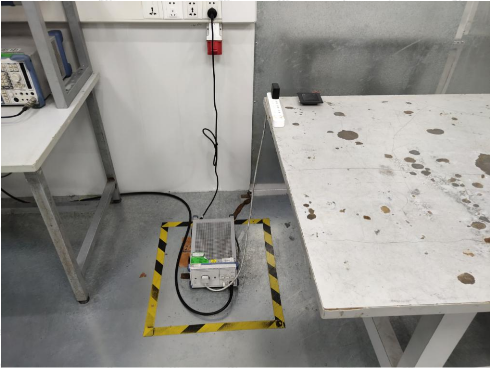
Photo of Power Line Conducted Emission Test
