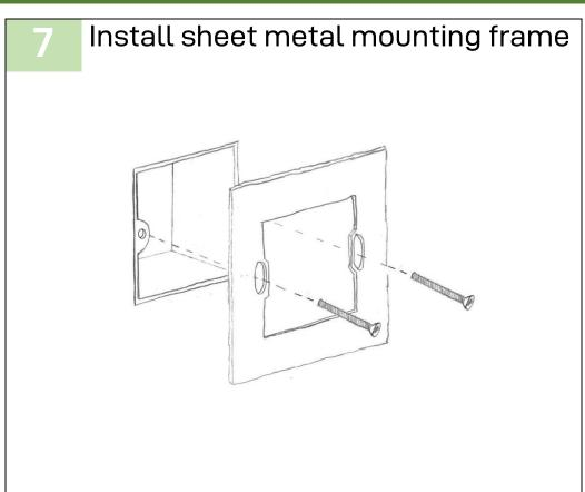
▲ Ensure that the mounting frame is level
