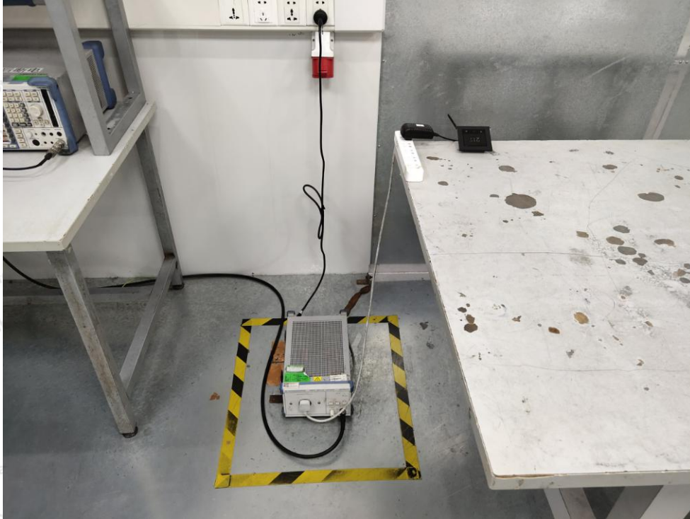
Photo of Power Line Conducted Emission Test
