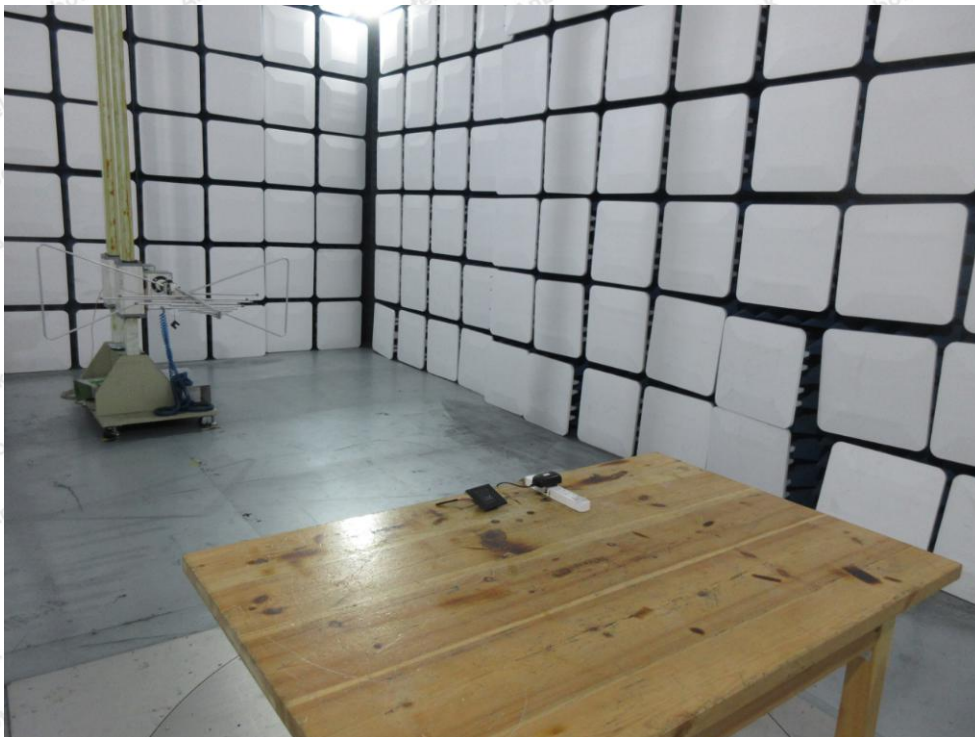
Photo of Radiation Emission Test
