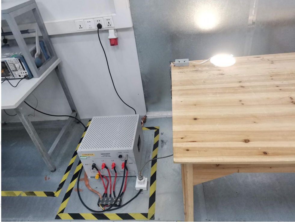
Photo of Conducted Emission Measurement
