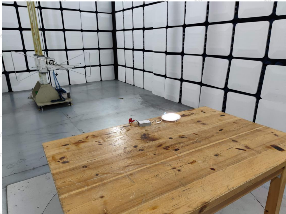
Photo of Radiation Emission Test
