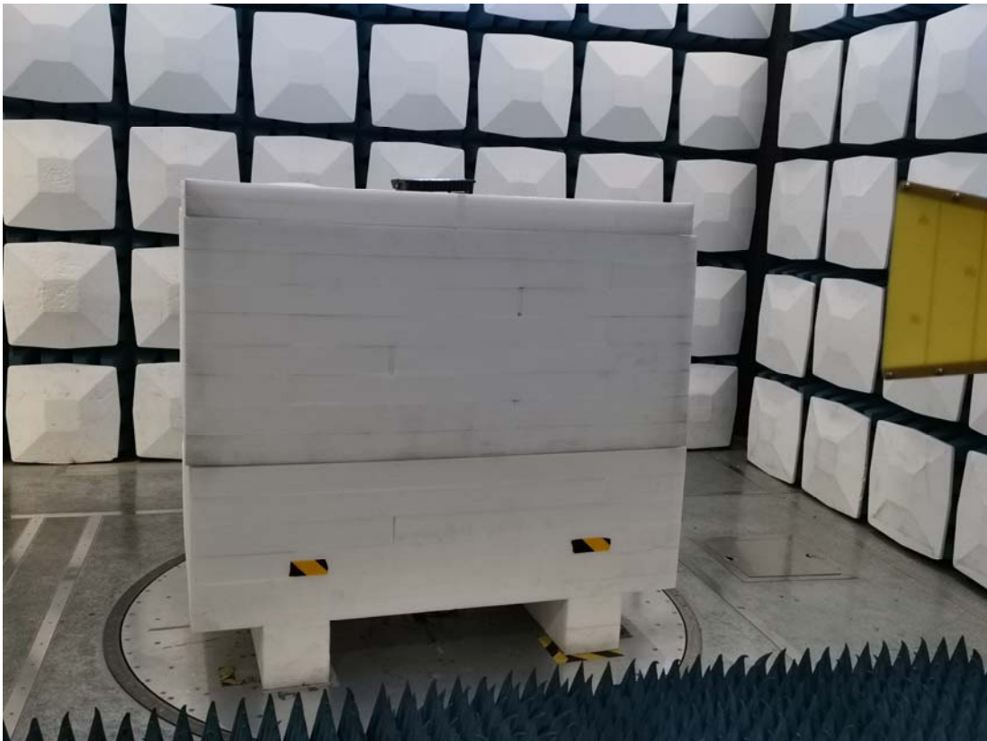
Radiated Emission Above 1GHz View
