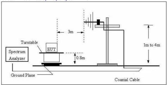
(C) Radiated Emission Test-Up Frequency Above 1GHz
