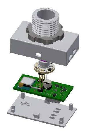
Assemble PCB assembly into housing as shown.
