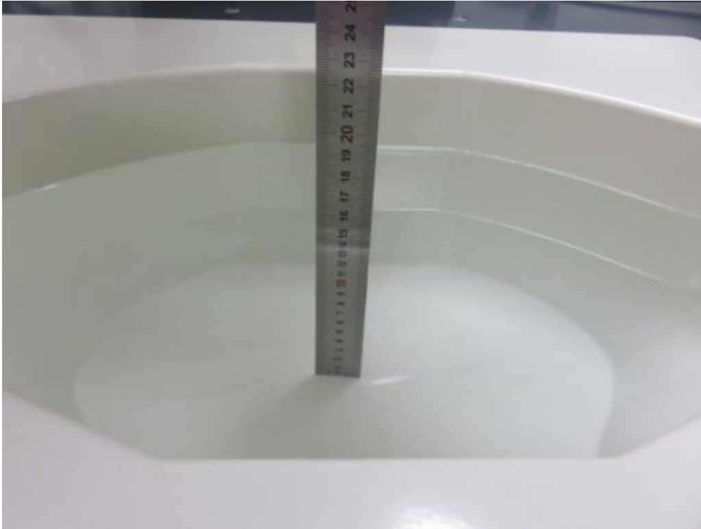
Photograph of the depth in the Body Phantom (3500-6000MHz, 15.3cm depth)
