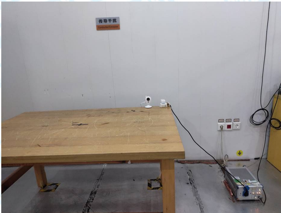
Photo of Setup for Conducted Emission
