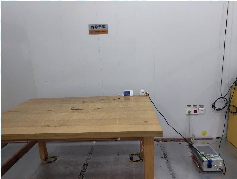
Photo of Setup for Conducted Emission
